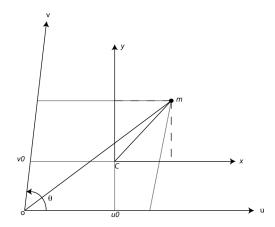
Figure 2.4: Camera Intrinsic Parameters
