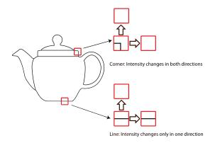
Figure 4.1: A Simple Corner Detection Algorithm
