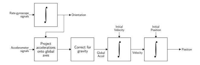
Figure 3.9: A Block-Diagram of A Strapdown IMU Algorithm, source [42]
