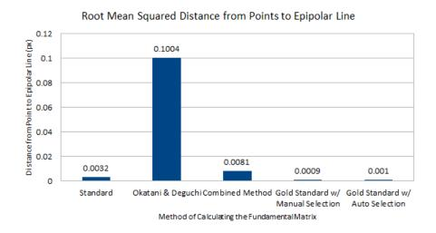
Figure 7.14: RMS Values for Distance from point to Epipolar Line - Image Set 3
