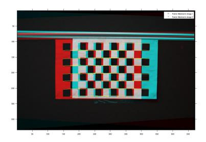
**Figure 7.5:** Point Match Candidates Determined from the Epipolar Constraint of the Rectified Images
