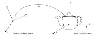
**Figure 2.3:** The Extrinsic Parameters of a Camera System. The origin of the Camera Coordinate System, C, is mapped to that of the World Coordinate System through Rotation R and Translation t.
