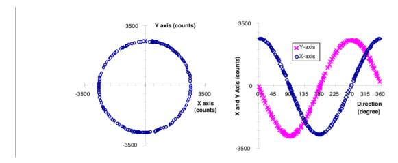
**Figure 3.7:** No Interference of Magnetometer Readings For 360°Rotation in Level Plane - Source [8]
