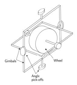
Figure 3.5: A Conventional Mechanical Gyroscope, taken from [47] in [42].
