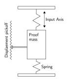
Figure 3.3: A Mechanical Accelerometer (Taken from [47] in [42] )
