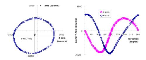
Figure 3.8: A Magnetometer Rotated Horizontally Around 360°Whilst Experiencing Interference from A Car Body and Engine - Source [8]
