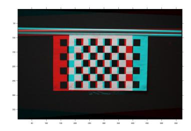
**Figure 7.4:** Image Set 1 Rectified with Rotation information obtained from the Orientation Sensor
