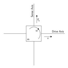
Figure 3.6: A Gyroscope Based on a Vibrating Mass
