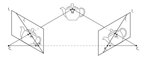
Figure 2.5: Epipolar Geometry
