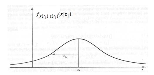
**Figure 3.10:** Conditional Probability Density of Position Based on Measured Value  $z_1$  - Taken from [40]
