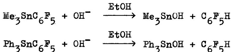
In the absence of ethanol, cleavage by alkali is very slow. This ready cleavage by nucleophilic reagents is a general property of fluorocarbon tin compounds, and is probably due to the high polarity of the bond between the metal and the fluorocarbon group.
