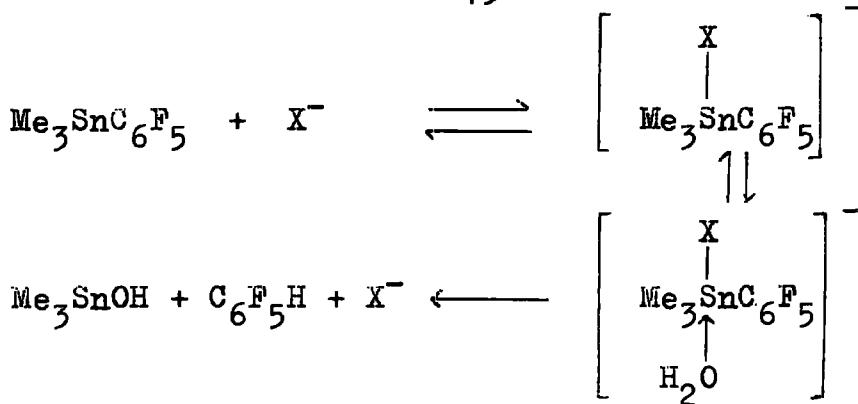
Direct replacement of pentafluorophenyl by fluoride ion, followed by hydrolysis, is ruled out by the fact that trimethyltin fluoride is not readily hydrolysed in aqueous solution.
