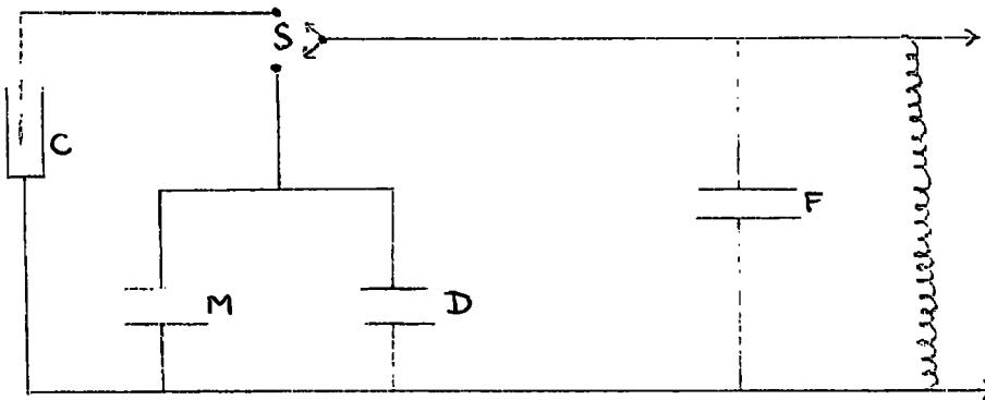
$C$  = the cell.  $S$  = switch for changing circuits.
