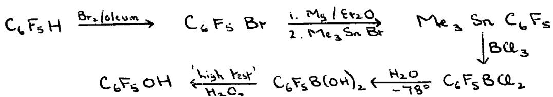
This reaction may provide a convenient route to substituted perfluorophenols, which cannot be prepared from the parent aromatic fluorine compound by the standard reaction with potassium hydroxide,<sup>107</sup> because of secondary reactions between the substituent and alkali.
