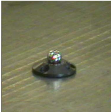
Figure 4.3 Visible red laser pointing to the surface of a tooling ball
