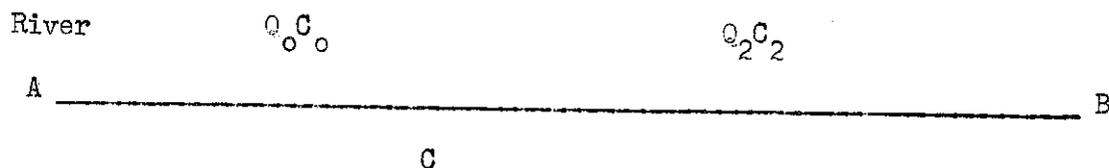
This schematic represents the mass balance of an effluent C, discharging into a river, AB.
