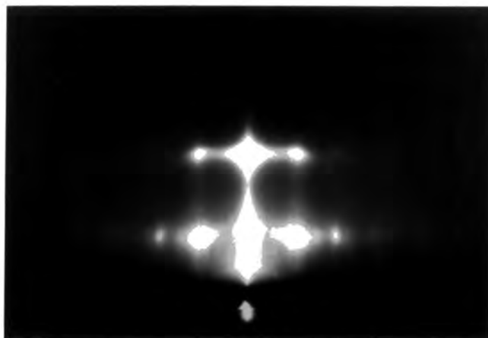
(c) Single crystal InP with 11 monolayers CdStearate ( \{100\} surface).
