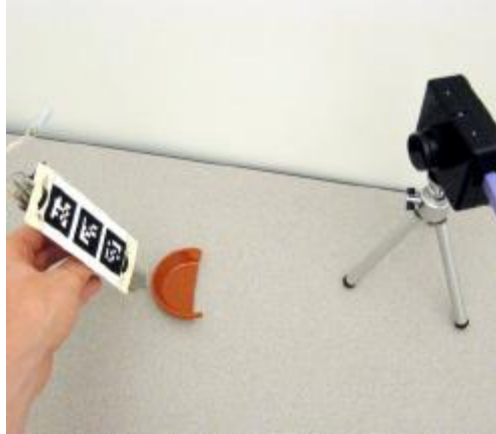
Figure 2.12: Physical surface acquisition of real-world 3D objects (Andrews and Lang 2007).
