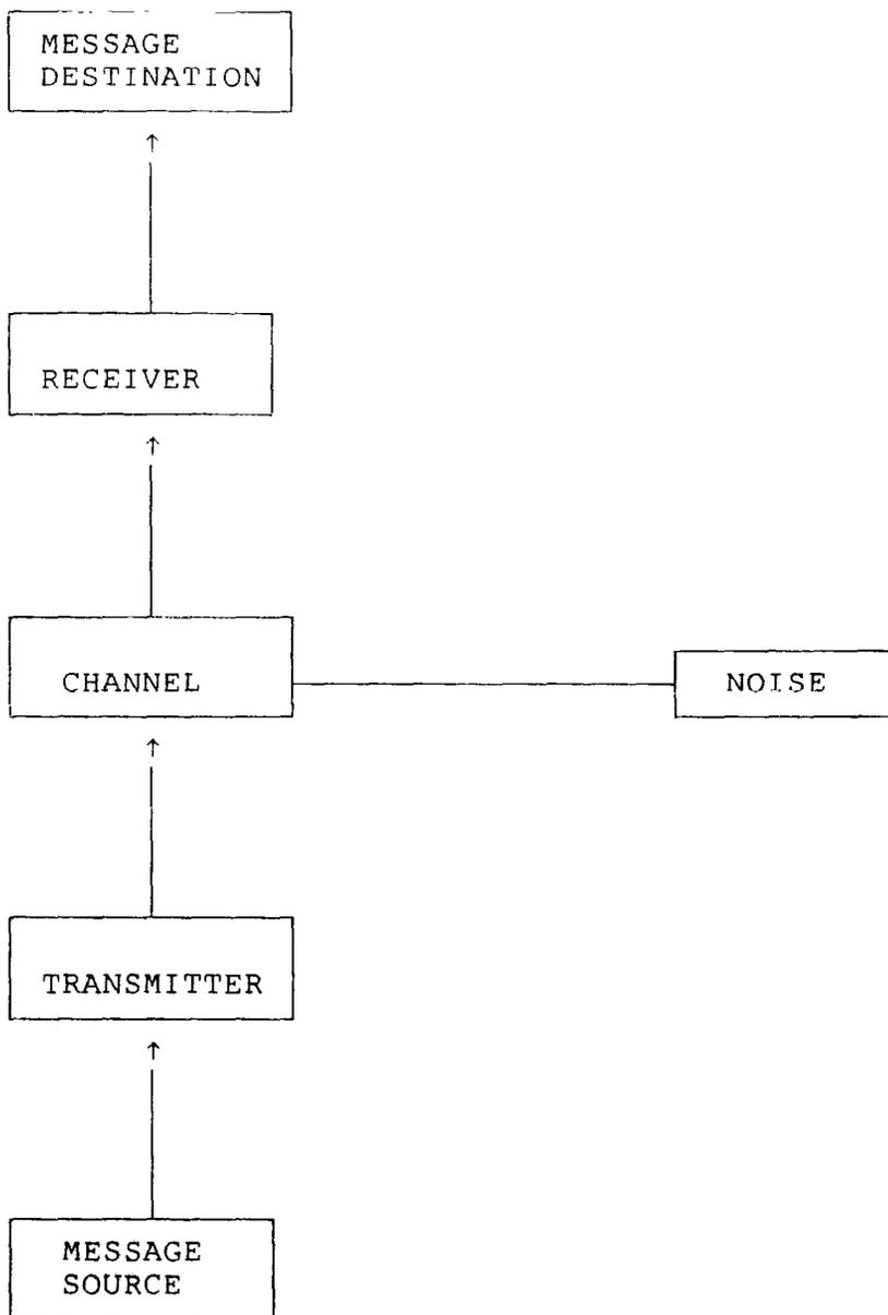
Figure 1.1 An engineer's model of the communication process (From C.E. Shannon and W. Weaver, *The Mathematical Theory of Communication*, University of Illinois Press, 1949)
