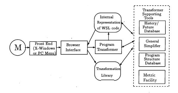
Figure 8.1: Design of the Prototype
