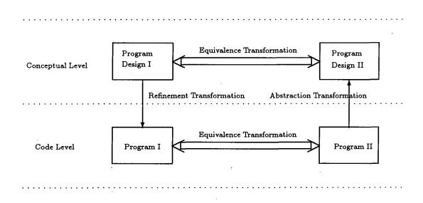
Figure 7.2: Three Types of Program Transformation
