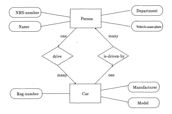
Figure 7.8: Deriving a Relationship from a Foreign Key
