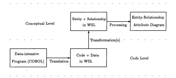
Figure 5.5: A Data Design Recovery Method
