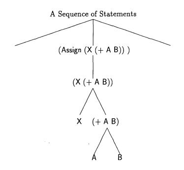
Figure 6.4: Diagrammatic Form of a WSL Syntax Tree
