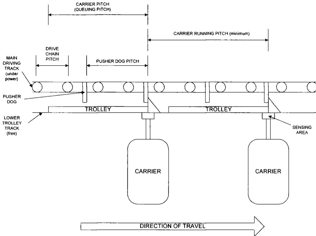
**Figure 10. General Power and Free System Configuration.**
