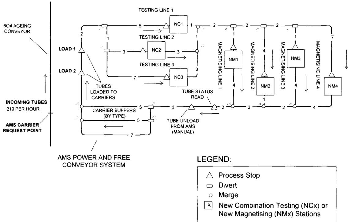
Figure A13. Schematic of Design Scenario 1 for AMS Circuit Layout.
