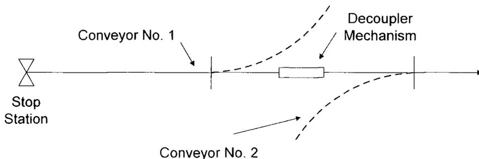
Figure 13. Decoupler Configuration.
