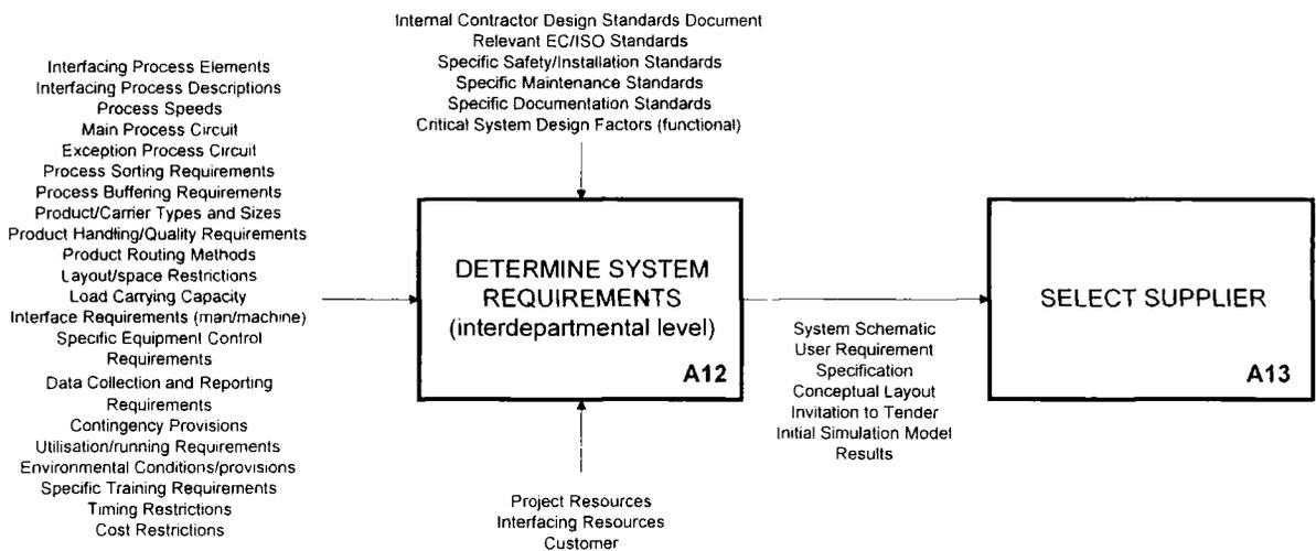
Figure 8. The Process of Determining System Requirements.
