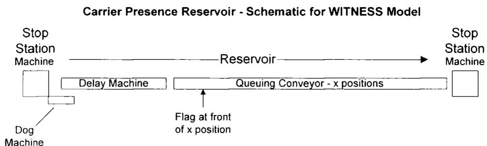
**Figure 33. Simulation Schematic for Carrier Presence Reservoir Model.**
