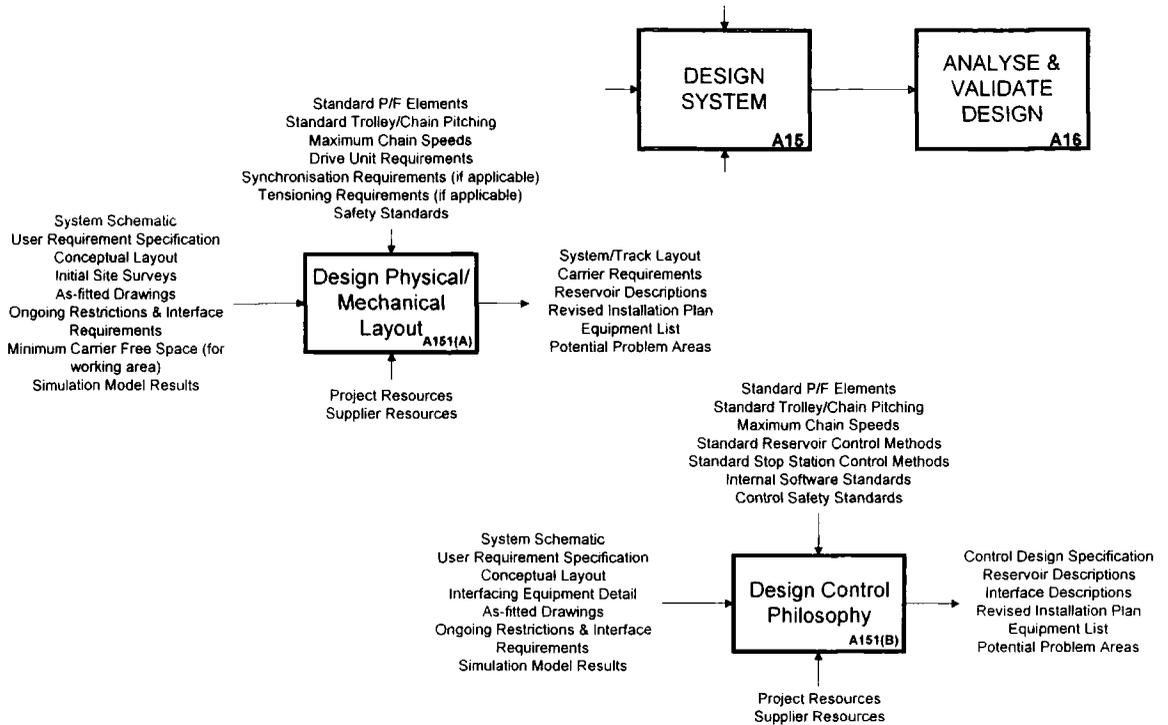
Figure 9. The Process of Designing the System.
