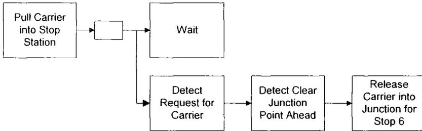
**Stop Station 21 - Stop after Testing Line and By-pass Lane, prior to Main Line**
