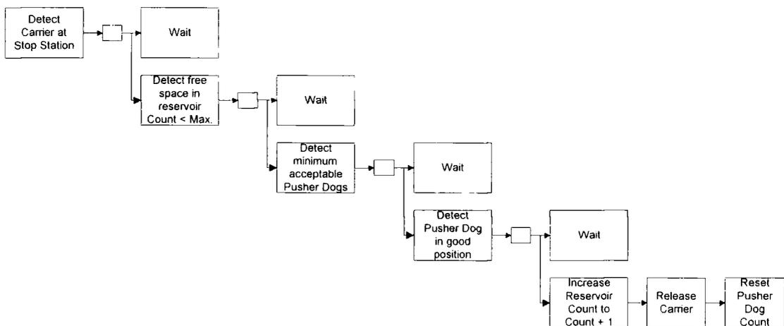
**Figure 36. Detailed Process Map for Counting Control.**
