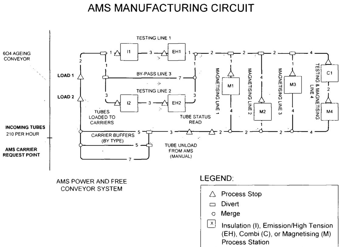
Figure 42. Schematic for the AMS Circuit.
