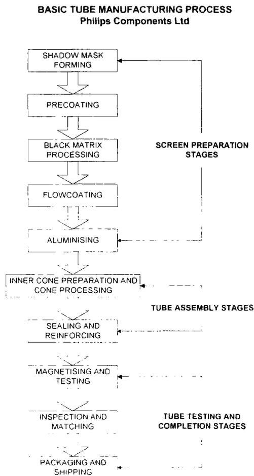
Figure 2. Tube Manufacturing Process
