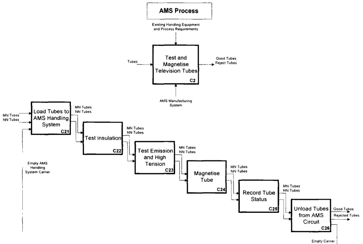
Figure 41. Process Map for the AMS Circuit.
