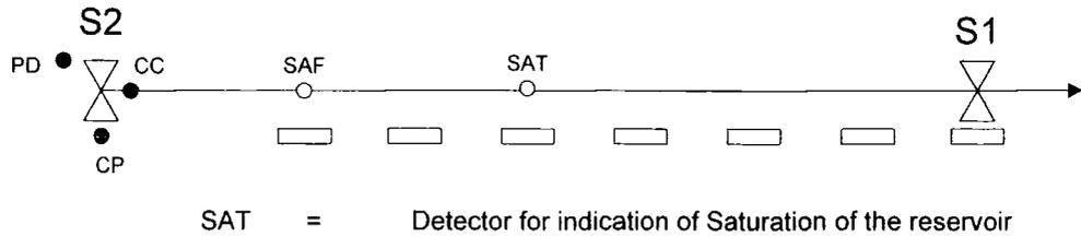
Figure 19. Reservoir Utilising Saturation Control.
