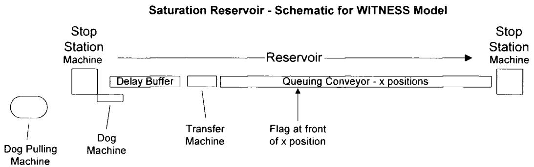
**Figure 37. Simulation Schematic for Saturation Reservoir Model.**
