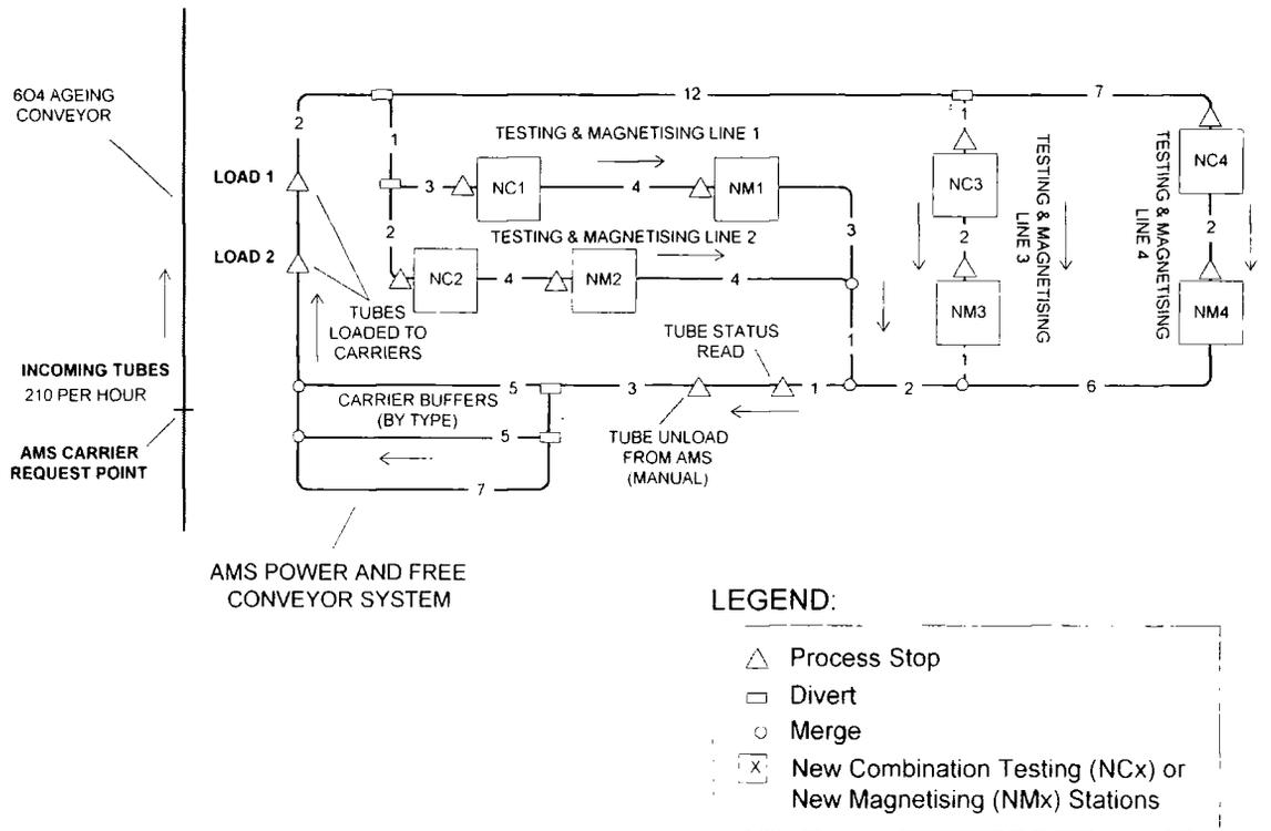
Figure A14. Schematic of Design Scenario 2 for AMS Circuit Layout.
