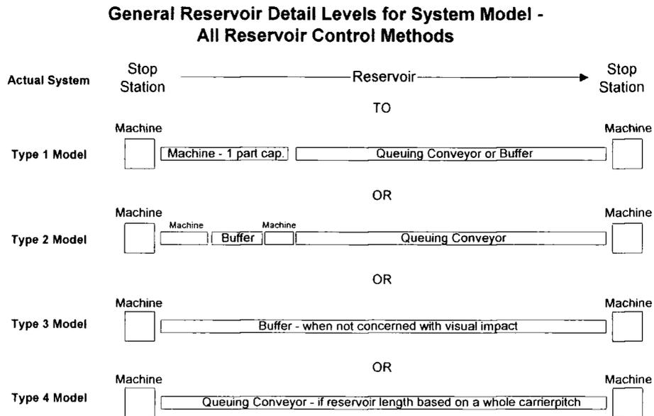
**Figure 39. Generic Simulation Schematics for System Level.**
