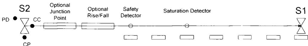
**Figure 28. Sensor Arrangement in Saturation Reservoirs.**
