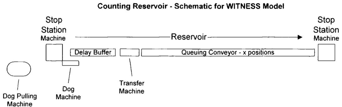
**Figure 35. Simulation Schematic for Counting Reservoir Model.**
