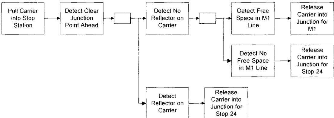
Figure 43. Example Structured Flow Diagrams for the AMS Handling System.
