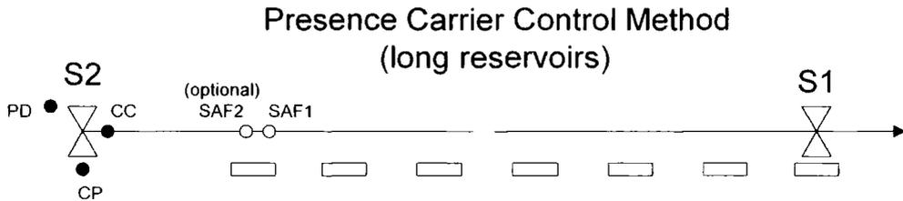
**Figure 27. Alternative Sensor Arrangement for Long Presence Carrier Reservoirs.**
