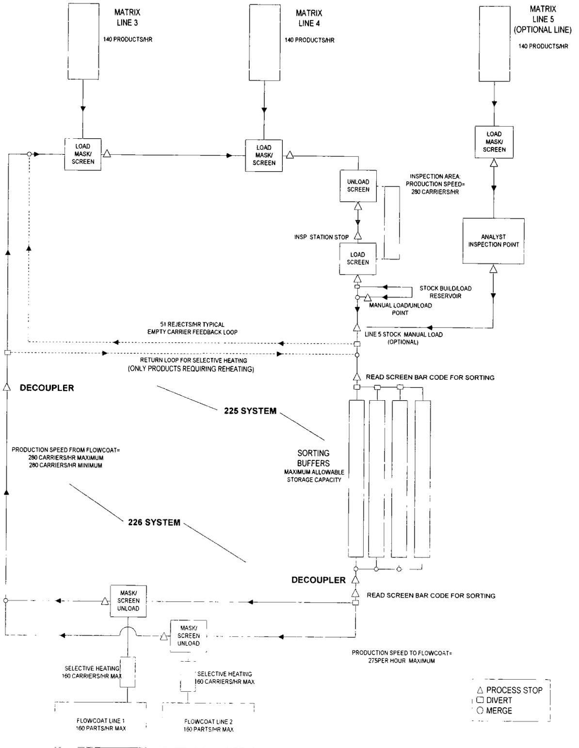
**Figure 40. Schematic for the 225/226 System.**
