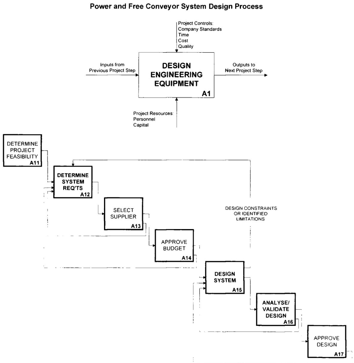
Figure 7. IDEF Map of the Power and Free Handling System Design Process.
