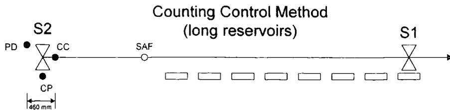
**Figure 29. Sensor Arrangement in Long Counting Reservoirs.**
