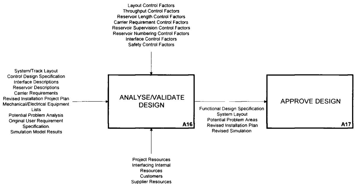
Figure 21. The Process of Analysing and Validating the Design
