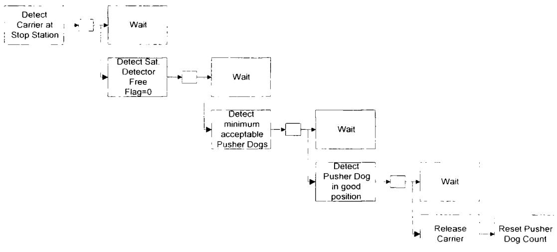
**Figure 38. Detailed Process Map for Saturation Control.**
