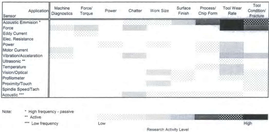
Fig. A.1 Summary of research activity in on-line cutting process monitoring [Byrne et al. 1995]
