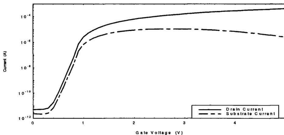
**Figure 3.2 Drain current and substrate current versus gate voltage for an nMOS transistor ( $W=1 \mu\text{m}$ ,  $L=0.8 \mu\text{m}$ ,  $V_{DS} = 5$  V, Process: EC/3 (see appendix D))**
