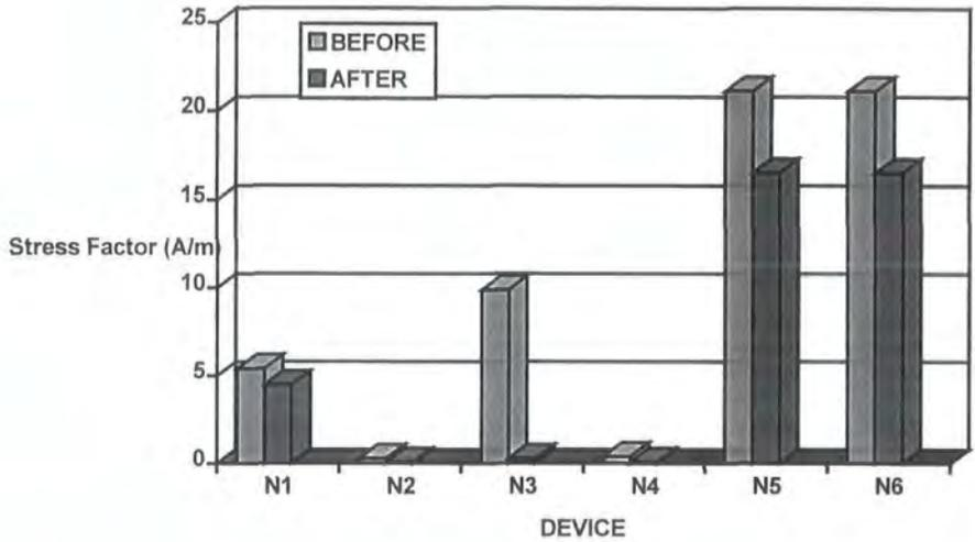
**Figure 7.3** Bar graph showing the stress levels on all the devices in DL1 before after swapping of N1 with N2 and N3 with n4. (Technology: EC/3, Device N: 1/0.8)
