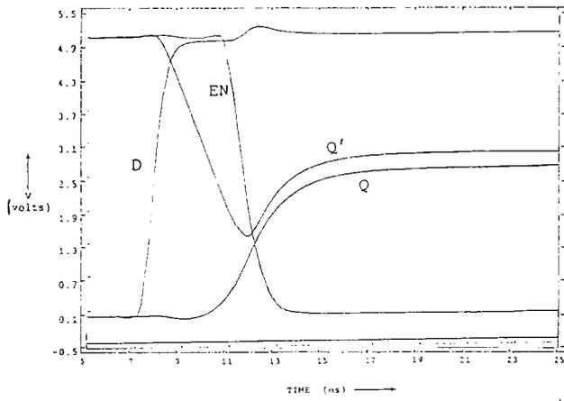
Fig 11. Metastability simulation for MX-GATE
