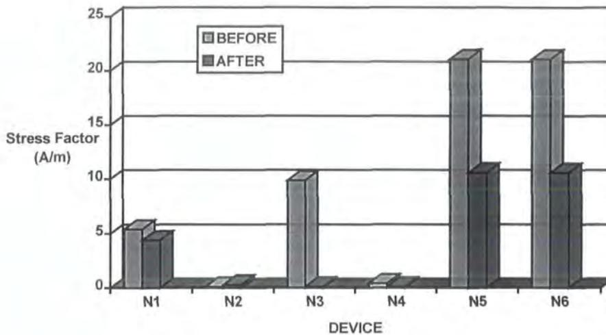
**Figure 7.5 Stress factors for devices in DL1 before and after all the improvements in the design.** (Technology: EC/3, New device dimensions are: N1, N2, N3, N4: W/L = 1/0.8 and N5,N6: W/L = 2/1.5 )
