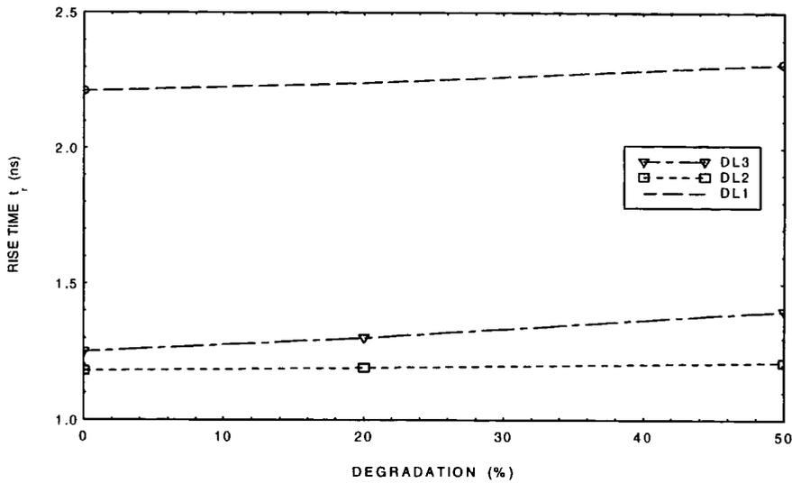
**Figure 5.10 Rise Time as a function of Degradation for the three latch circuits**
