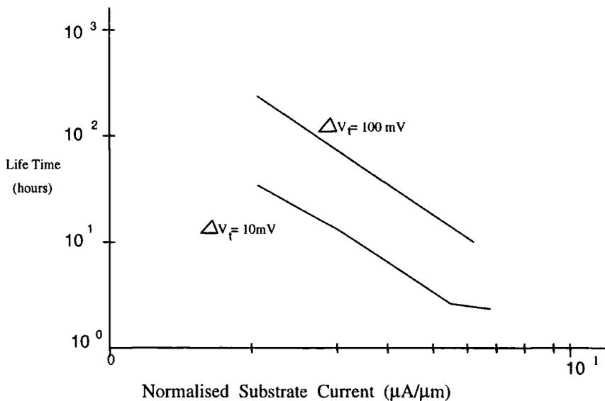
**Figure 3.9 Lifetime vs normalised substrate current: HOTRON model**
