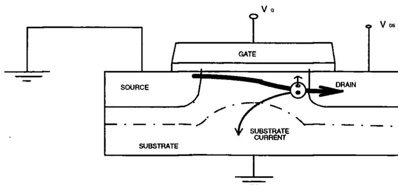
**Figure 3.1 Cross section of an nMOS transistor showing substrate current generation**
