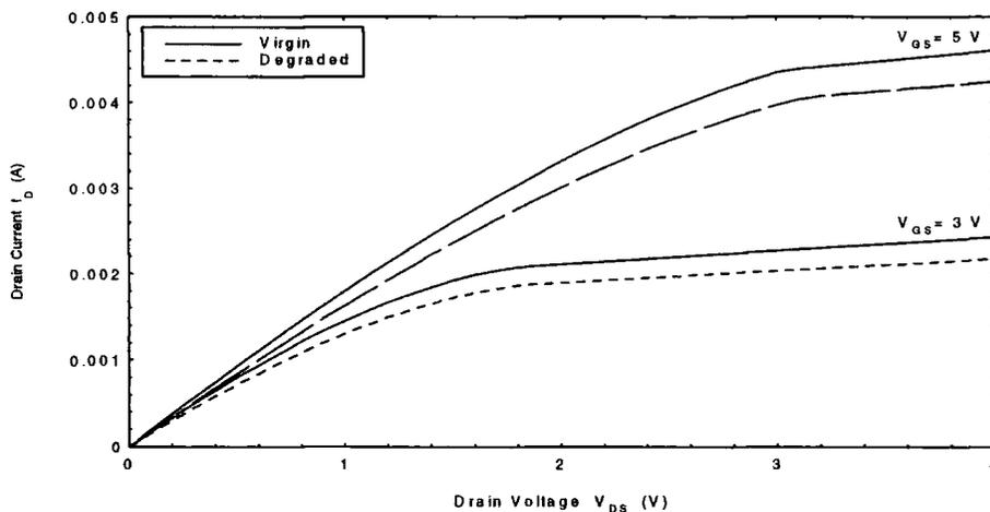
**Figure 3.13 Characterisation of degradation effects:  $I_D$  vs  $V_{DS}$  plotted for a virgin device and for a device with SPICE parameters degraded by 10% (Device: N:10/0.55, Process: EC/3 ) Lunenburg [3.41].**
