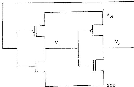
Fig 3. Transistor level circuit for the latch
