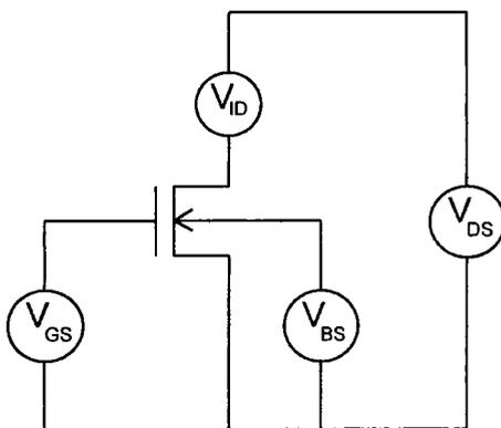
MOSFET CHARACTERISTICS NMOS  $I_D - V_{DS}$
