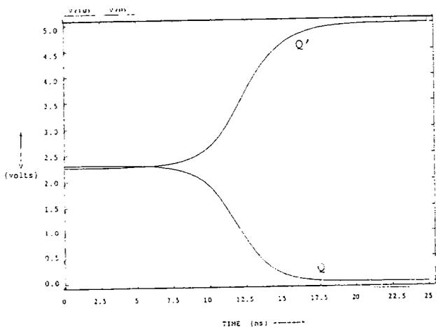
Fig 7. Metastable operation of a nearly matched latch
