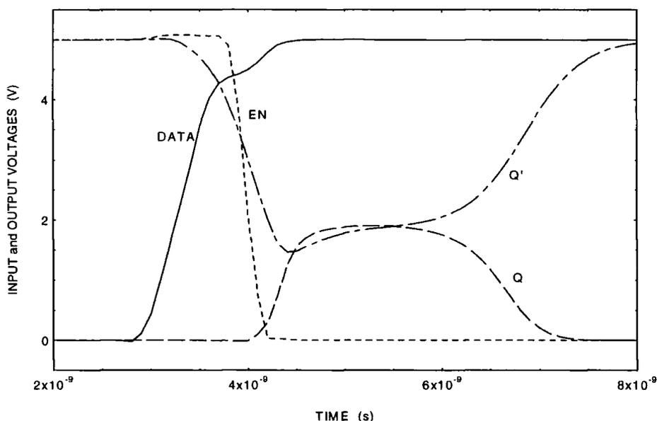
**Figure 6.7** Metastability simulation for latch DL3 at a clock edge of 0.7139798 ns.
