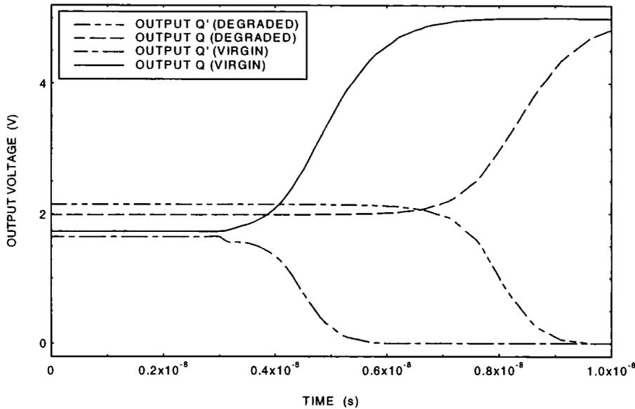
**Figure 6.11 Resolving time simulations with and without degradation for DL1.**
