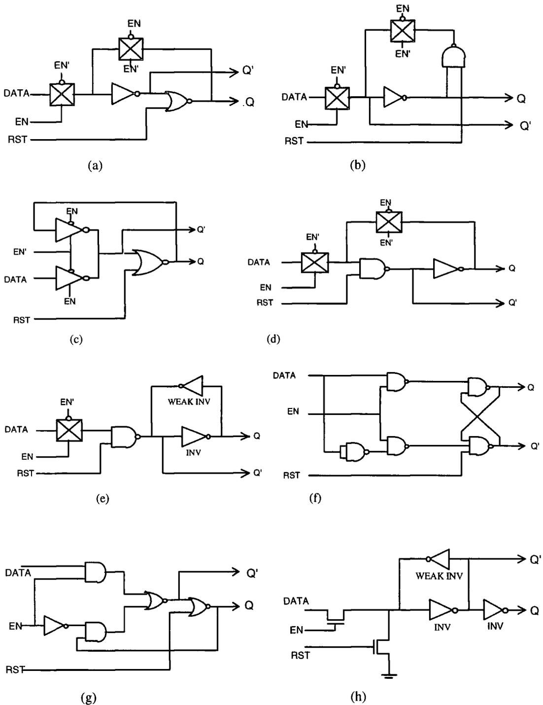
**Figure 4.1 D-latch circuits**
