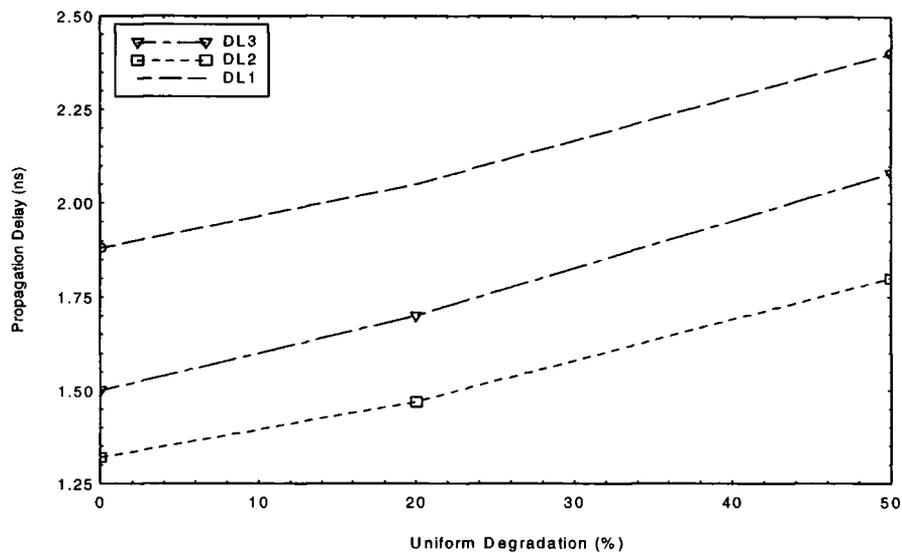
**Figure 5.12 Propagation Delay Vs Degradation for the latch circuits**
