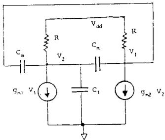
Fig 4. Small signal model of the latch
