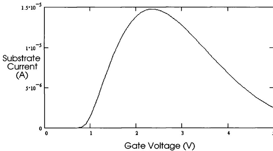
**Figure 3.4 Substrate current plotted using Sakurai model**
