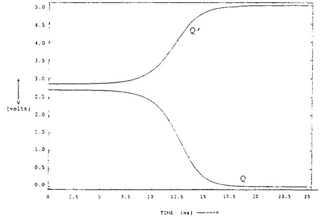
Fig 12. Metastability resolving for MX-GATE
