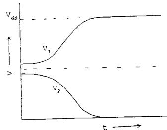
Fig 6. Voltage evolution at outputs of latch
