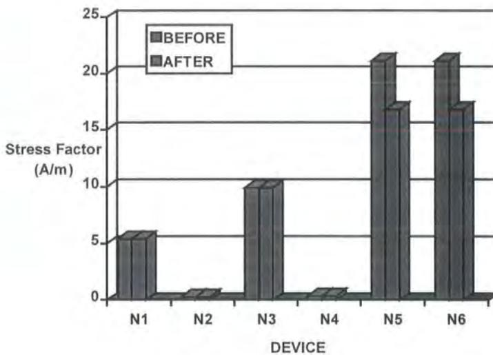
**Figure 7.4** Stress levels for devices in DL1 before and after doubling of the channel widths for N5 and N6. (Technology: EC/3, New device dimensions are: N1, N2, N3, N4: W/L = 1/0.8 and N5,N6: W/L = 2/0.8)
