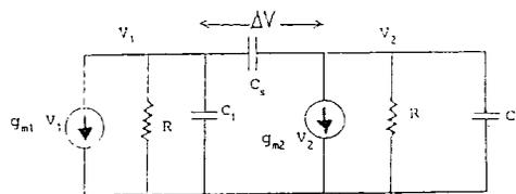
Fig 5. a.c. equivalent circuit of the latch
