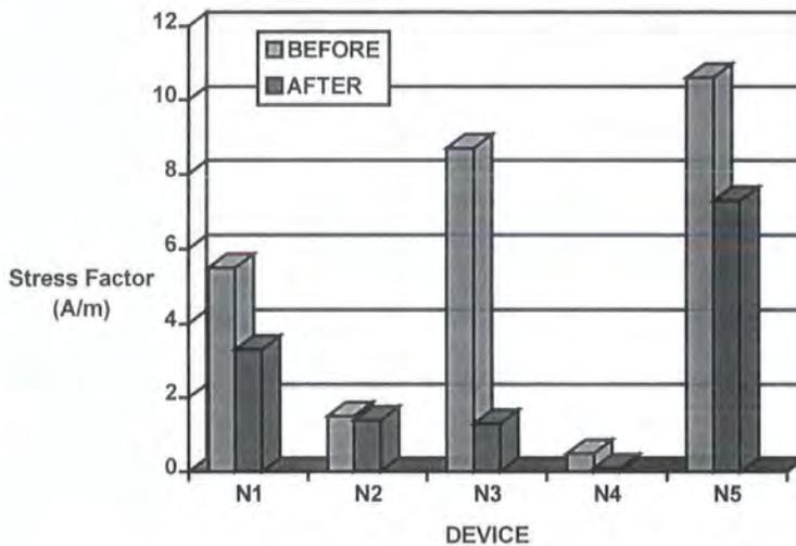
**Figure 7.7 Stress factors for DL3 before and after design changes**
