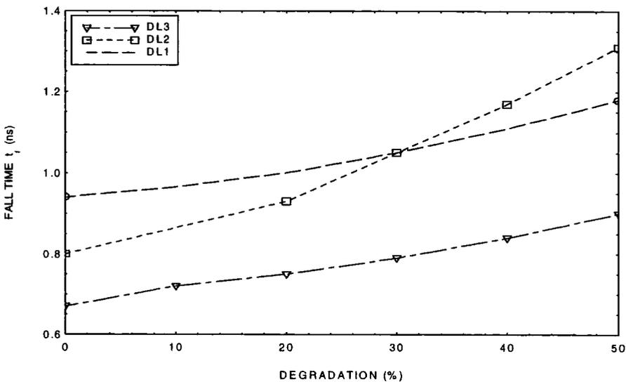
**Figure 5.10 Fall Time as a function of Degradation for the three latch circuits**
