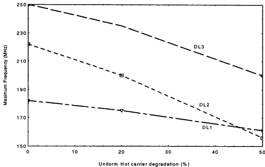
**Figure 5.15 Max. frequency Vs uniform degradation plotted for the latch circuits**
