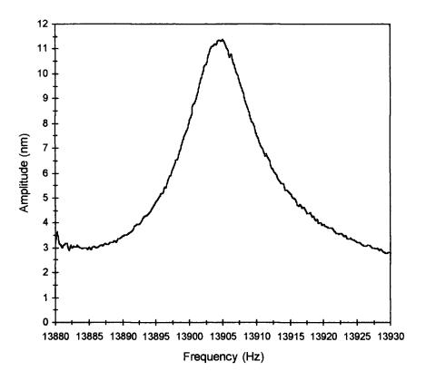
Figure 8.6a. Frequency response of fourth mode.
