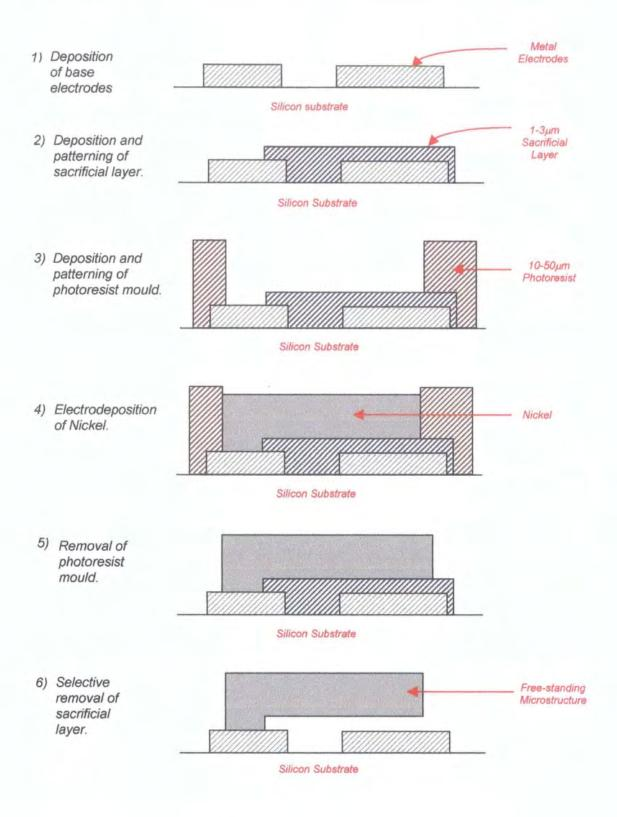
Figure 4.1. Production of nickel microstructures.
