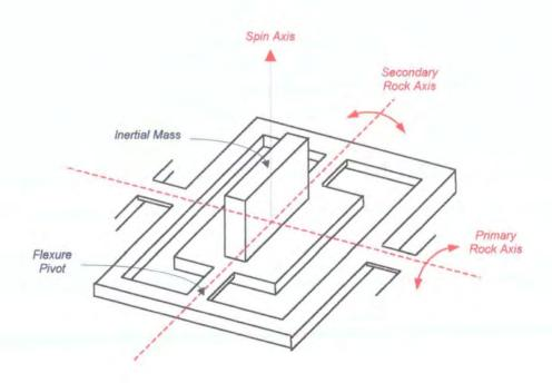
Figure 6.13. Gimballed frame vibratory gyroscope.
