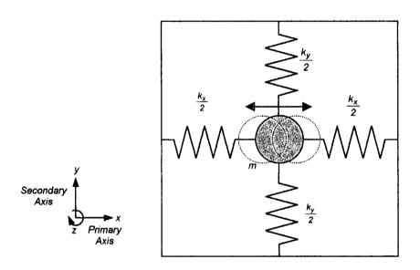
Figure 6.2. General model of a vibratory gyroscope.
