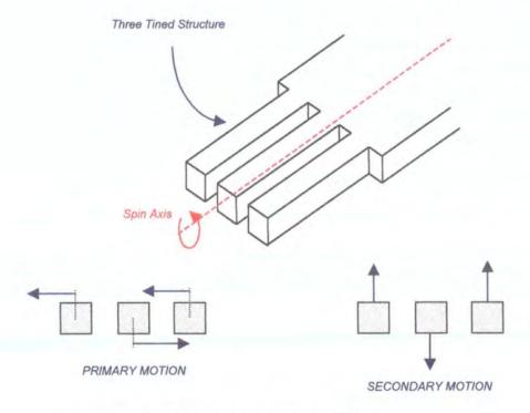
Figure 6.7. Trident Tuning Fork Arrangement.
