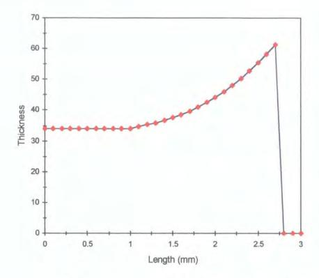
Figure 3.7. Typical thickness profile of a 2.7mm x 500μm cantilever.
