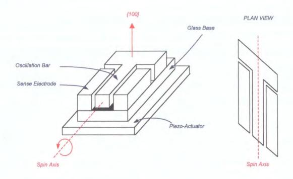
Figure 6.12. Micromachined vibrating beam gyroscope.
