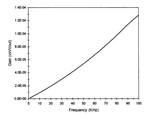
Figure 8.17. Electrical coupling between drive and detection circuitry.
