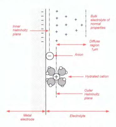
Figure 3.1. Electrical double layer.
