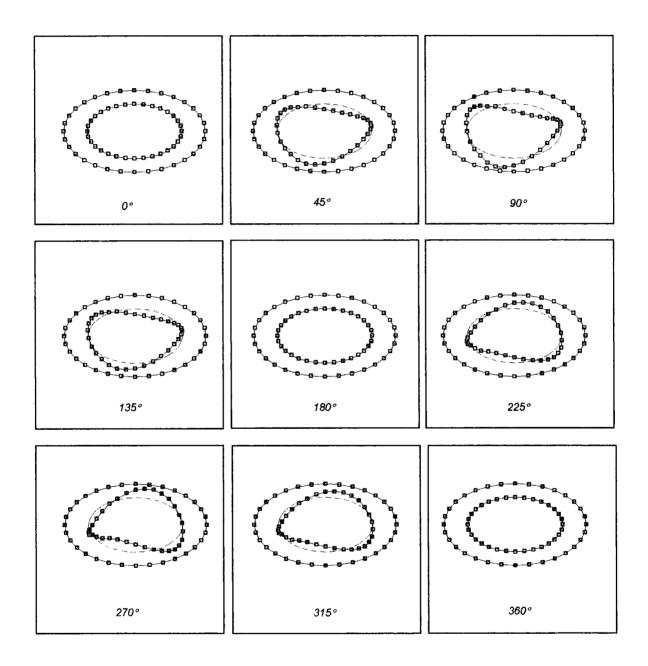
Figure 8.15. Still frame animation of fourth out-of-plane mode shape
