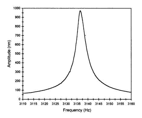
Figure 5.12. Amplitude response of 2.7mm cantilever.
