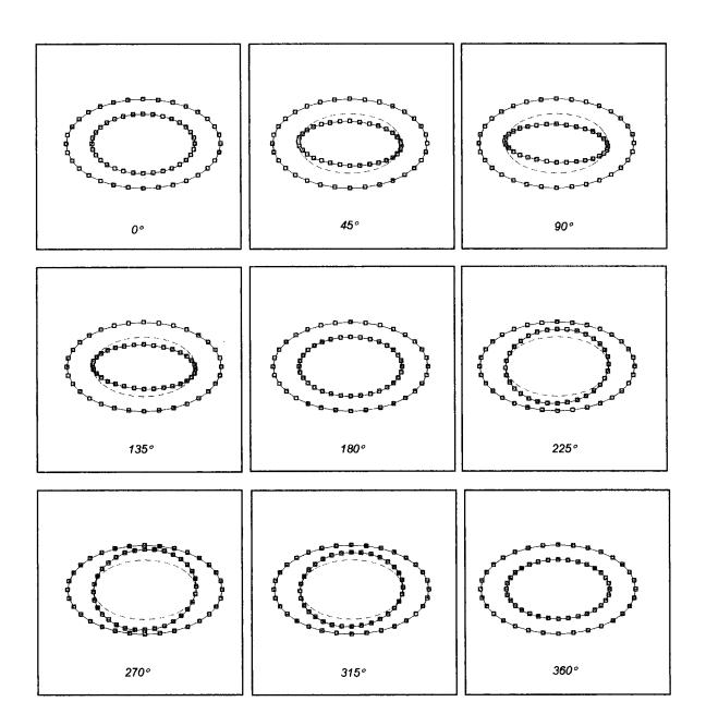
Figure 8.14. Still frame animation of third out-of-plane mode shape.
