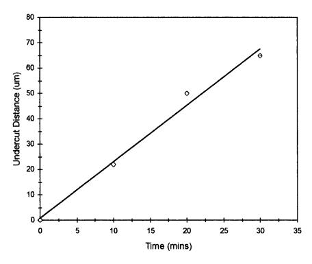
Figure 4.14. Determination of lateral titanium etch rate for a 3μm layer in 10% HF solution.
