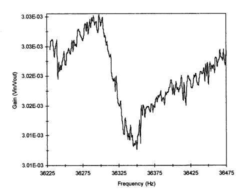
Figure 8.22a. Magnitude response at 270° detection electrode.
