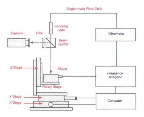
Figure 5.4. Experimental measurement system.
