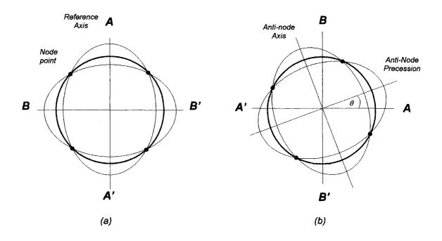
Figure 7.3. Precession of the standing wave vibration pattern.
