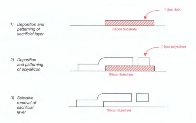
Figure 2.5. Surface micromachining.
