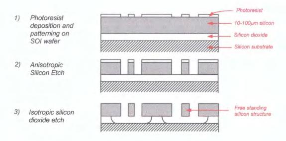
Figure 2.8. SOI process concept.
