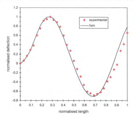
Figure 5.19. Third flexural modeshape of the 2.7mm cantilever beam.
