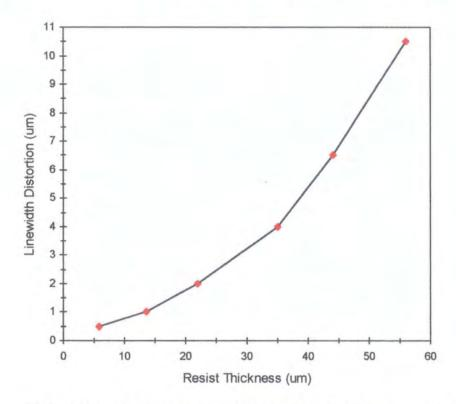
Figure 4.8. Relationship between thickness and typical linewidth distortion.
