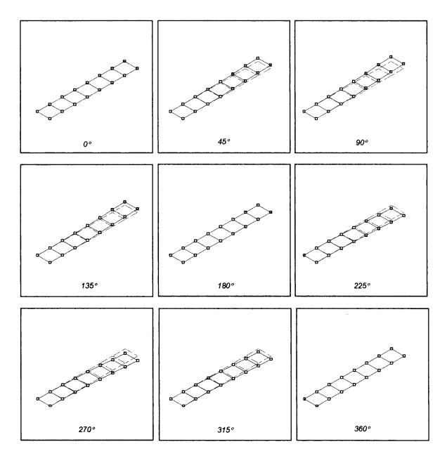
Figure 5.20. Still frame animation of first flexural mode of vibration.
