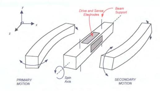
Figure 6.3. Operation of a vibrating beam gyroscope.
