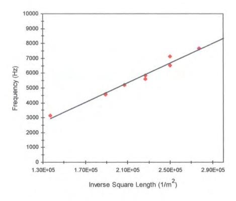
Figure 5.25. Resonant frequency and inverse square of length.
