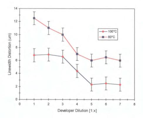
Figure 4.9. Influence of developer dilution on linewidth deviation.
