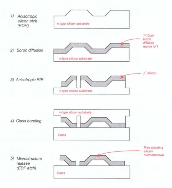
Figure 2.4. Dissolved wafer fabrication technique.
