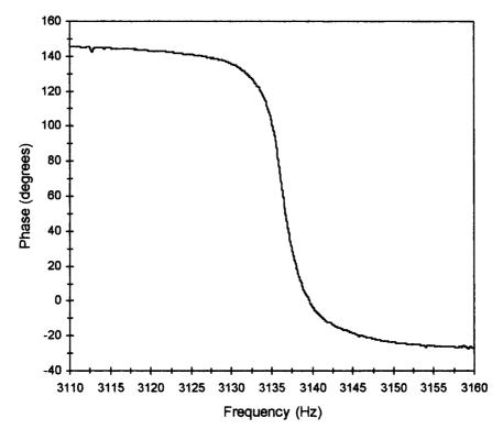
Figure 5.13. Phase response of the cantilever.
