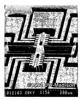
(c) Electrostatic resonator.
