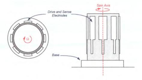
Figure 6.10. A typical cylinder gyroscope.
