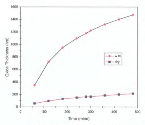
Figure 4.2. Wet and dry oxidation growth curves.
