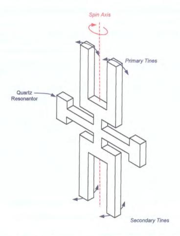
Figure 6.6. Operation of the Systron Donner GyroChip.
