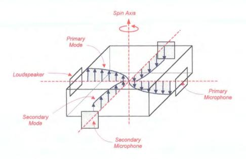
Figure 6.16. Concept of the Acoustic gyroscope.
