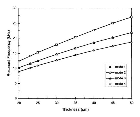
Figure 7.9. Influence of structural thickness on resonant frequency.
