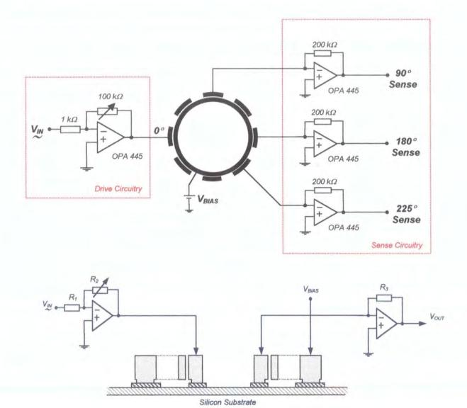
Figure 8.16. Electrical operation of the ring gyroscope.
