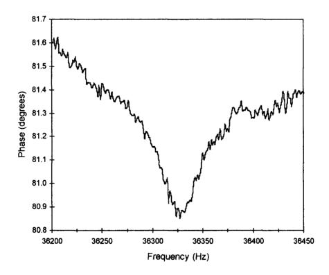
Figure 8.21b. Phase response at 90° detection electrode.
