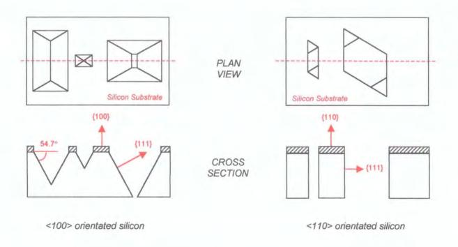
Figure 2.1. Crystallographic etching of Silicon.
