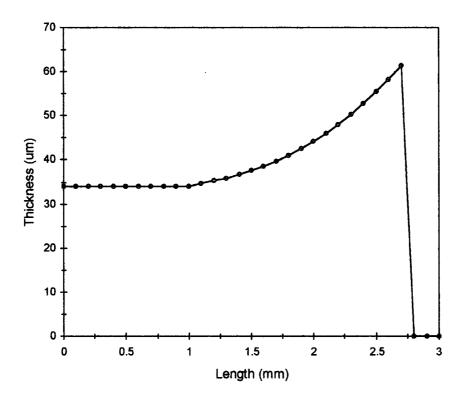
Figure 5.6. Thickness profile of the 2.7mm long cantilever beam.
