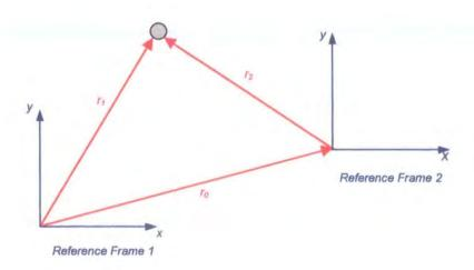
Figure A. Determination of position from different frames of reference.
