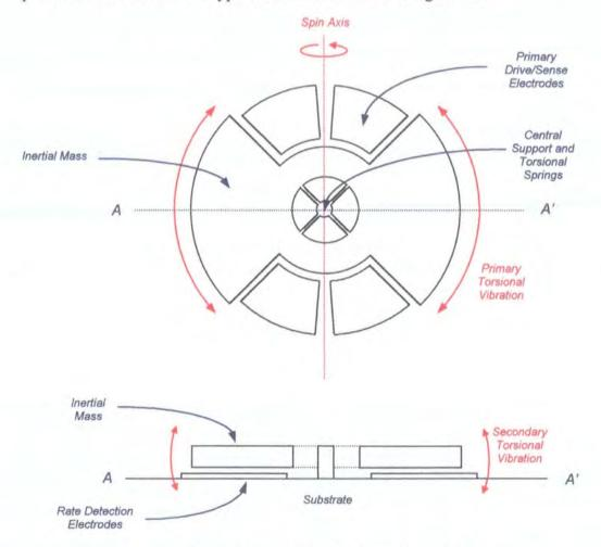
Figure 6.15. Torsional resonator gyroscope.
