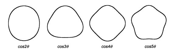
Figure 7.2. Resonant mode shapes of a uniform ring.
