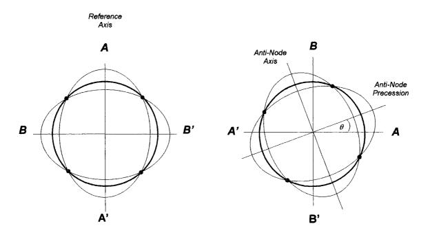
Figure 6.8. Operation of a shell type vibratory gyro.
