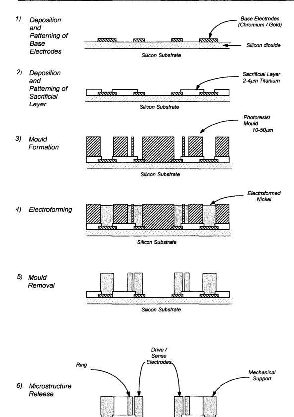
Figure 8.1 Fabrication of nickel ring gyroscopes.
