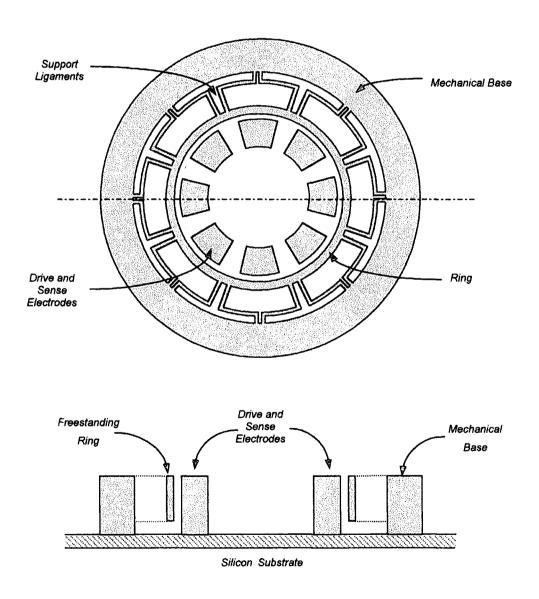
Figure 7.6. Schematic diagram of the micromechanical nickel ring gyroscope.
