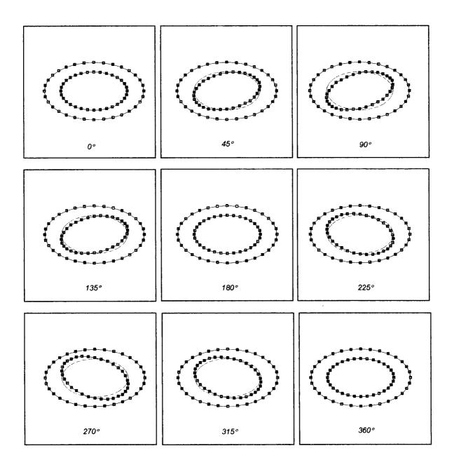
Figure 8.13. Still frame animation of second out-of-plane mode shape.
