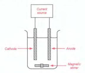
Figure 3.2. Electrolytic cell design.
