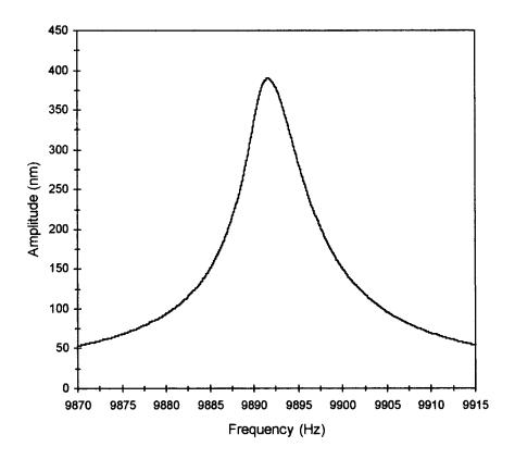
Figure 8.4a. Frequency response of first flexural mode shape.
