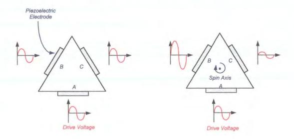
Figure 6.4. Operation of Murata's GyroStar.
