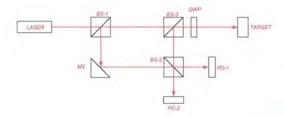
Figure 5.2. Modified Mach-Zehnder Interferometer.
