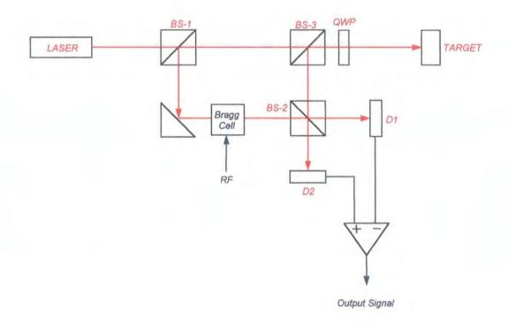
Figure 5.3. Laser vibrometer configuration.
