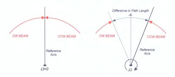
Figure 6.1. Operating principle of an optical gyroscope.
