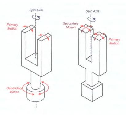
Figure 6.5. Operation of tuning fork gyroscopes.
