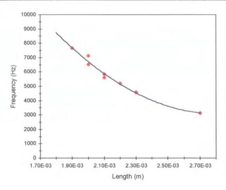
Figure 5.24. Variation of resonant frequency with beam length.
