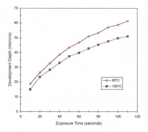
Figure 4.6. Development Depth as a function of exposure time.
