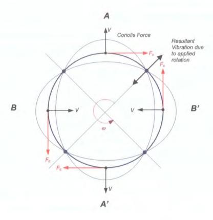
Figure 7.4. Generation of the secondary vibration.
