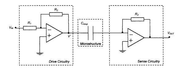
It can be shown that the output  $(V_{OUT})$  and input  $(V_{IN})$  are electrically coupled through the microstructure  $(C_{coup})$  and the output is directly proportional to frequency of the input:
