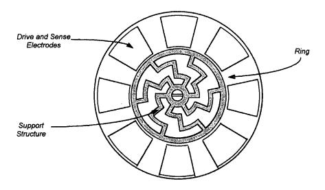
Figure 6.11. The British Aerospace VSG 2000 ring gyroscope.
