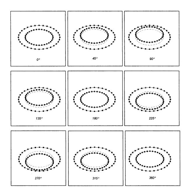
Figure 8.12. Still frame animation of first out-of-plane mode shape.
