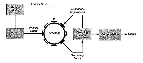
Figure 7.5. Practical operation of the ring gyroscope.
