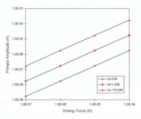
Figure 7.24. Amplitude vs. drive force for different levels of damping.
