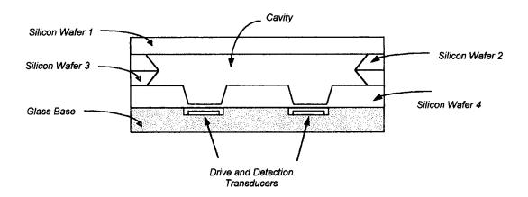
Figure 6.17. Cross-section through a silicon micromachined acoustic gyroscope,
