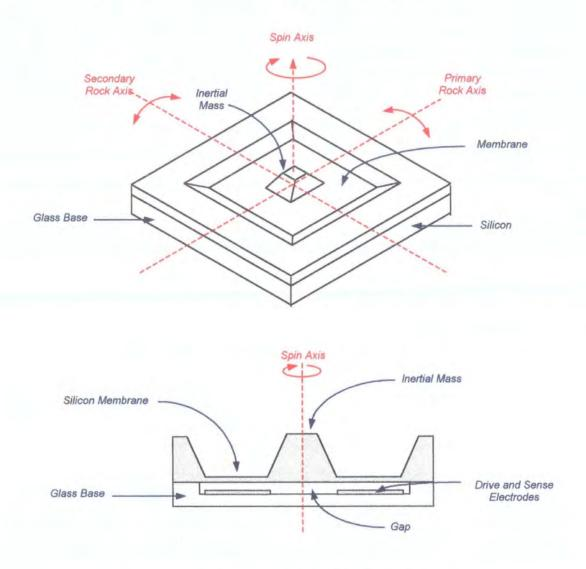
Figure 6.14. Schematic of the plate gyroscope.
