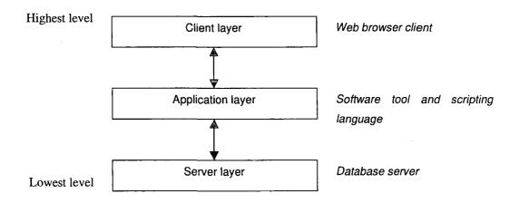
Figure 6.1: Layered system architecture model
