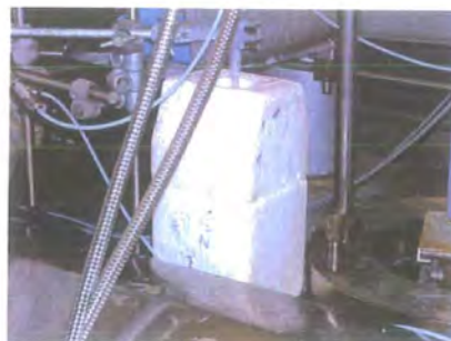
Fig 7 (cover the trap by a polystyrene box)
