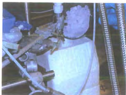
Fig 8 (fill the box with dry ice)
