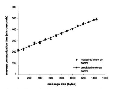
Figure 5-3 Measured and Predicted One-way Communication
