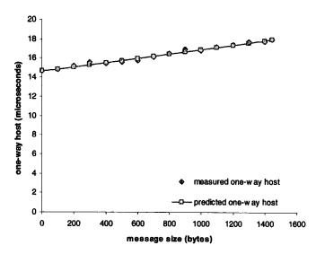
Figure 5-2 Measured and Predicted One-way Host Processing
