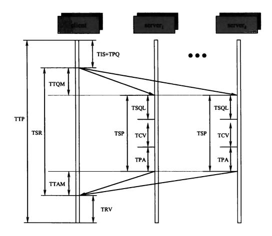
Figure 5-1 A Timing Diagram for ATIR Services
