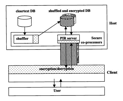
Figure 2-3 An Architectural Overview of Hardware-based PIR Schemes
