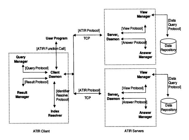
Figure 4-2 An ATIR System Architecture in a Replication Setting
