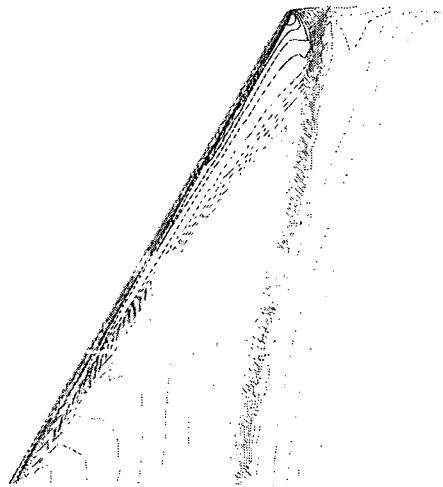
Figure 8.19 Mach number contours on the wing surface
