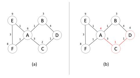
Figure 2.4: A\* process, (a) Initial state, (b) Final state
