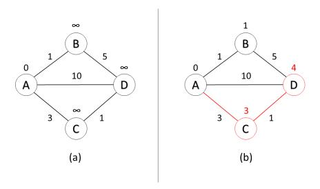
Figure 2.3: Dijkstra process, (a) Initial state, (b) Final state
