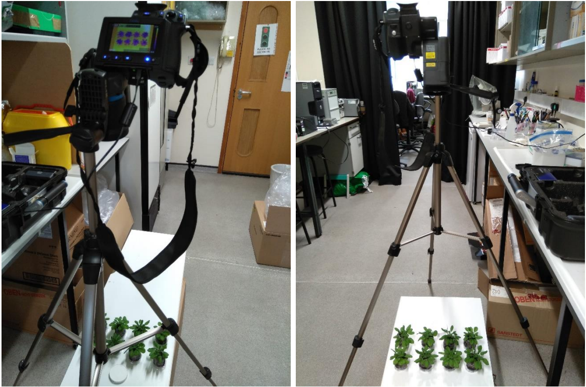
Figure 2.3: Experimental set-up for the thermal imaging of droughted plants in plugs. Plants were imaged under constant light, with or without water, with images taken every 30 minutes.
