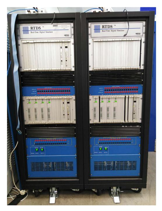
Figure 6.1: RTDS system at Durham University Smart Grid Lab.
