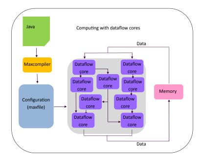
Figure 2.5: A dataflow program executing [94], indicating the streaming nature of computation and programming in space paradigm.
