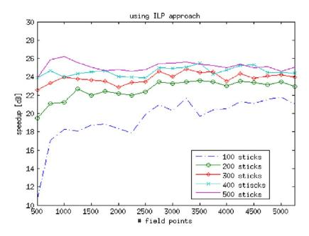
Figure 1.12: Speed-up of MISTIC code on a GPU compared to a CPU where Speedup<sub>dB</sub> =  $20 * log_{10}(t_{CPU}/t_{GPU})$  [69]. The sticks discretize a conductor in an active coil, e.g. Central Solenoid coil.
