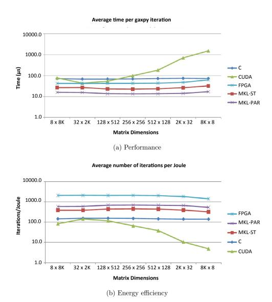
Figure 2.7: Comparison of BLAS Level 2 on CPU, GPU and FPGA in terms of (a) performance and (b) energy efficiency [102]. The GPU has the worst performance particularly for larger problem sizes, and the worst energy efficiency. This is due to the system and driver overhead for short and fat matrix dimensions and short vector effects for long and thin matrices. The FPGA has better performance and is by far the most energy efficient.
