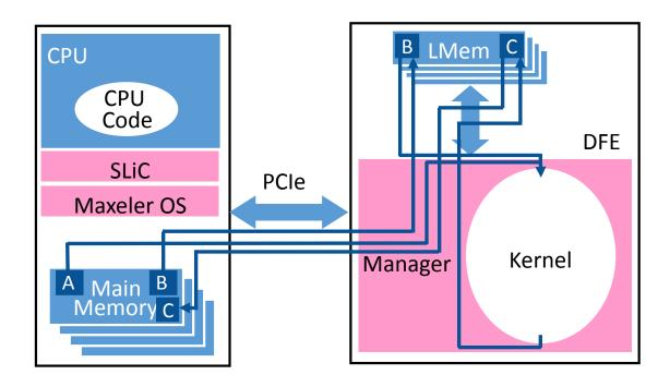
Figure 5.2: Schematic showing the data movement of the matrices A, B and result C between the CPU, DFE LMem and kernel.
