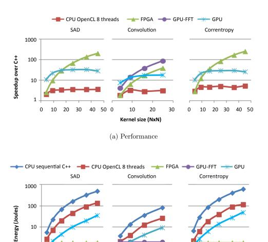
Figure 2.8: Comparisons of (a) performance and (b) energy efficiency tested on 720p images on CPU, GPU and FPGA [103]. The FPGA implementations have the highest acceleration whilst being the most energy efficient.
