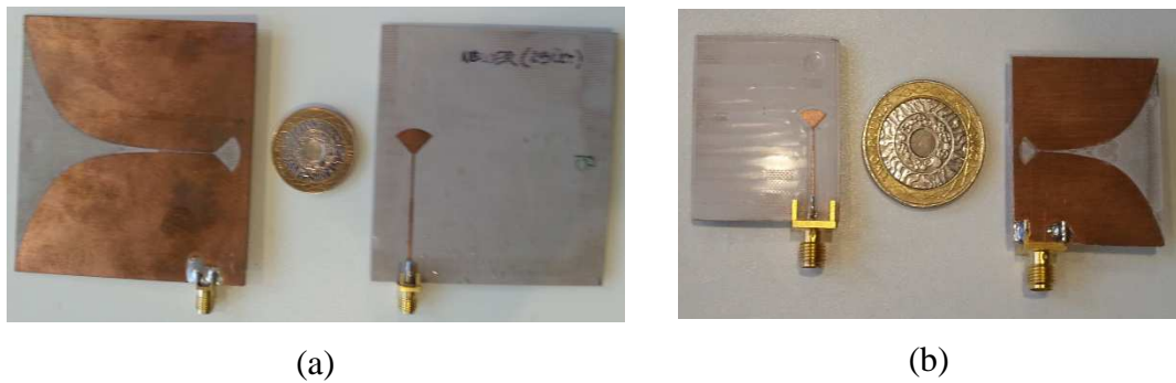
Figure 5.18: The front and back view of the fabricated antennas, (a) TSA-A; (b) TSA-B.
