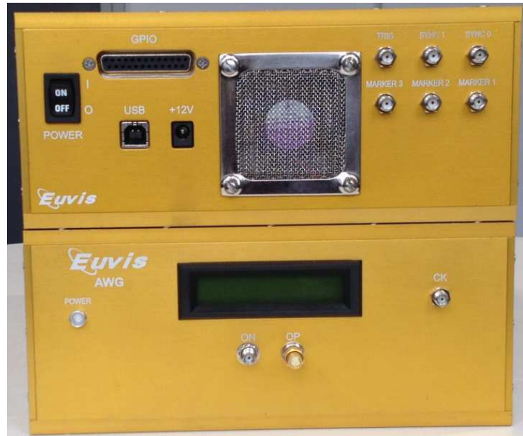
Figure 5.3: Back and front view of the Euvis AWG.
