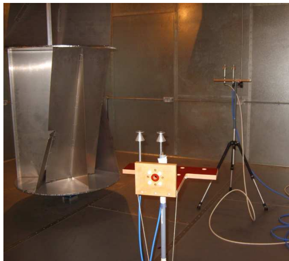
Figure C.1: Line of sight 2x2 MIMO configuration in the reverberation chamber
