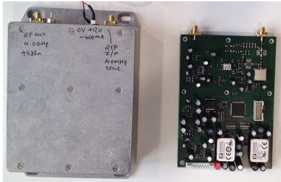
Figure 5.11: PLL and up-converter unit (left) in its metallic enclosure, (right) the unit circuit board.
