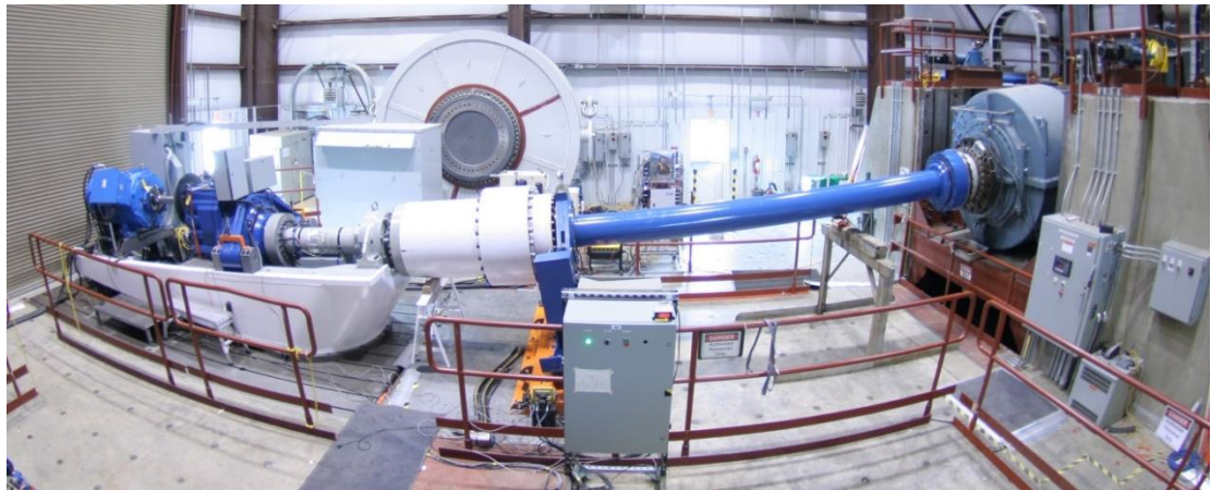
Figure 6.3: NREL dynamometer test stand with the 750 kW gearbox installed, photograph by Lee Jay Fingersh/NREL 16913.
