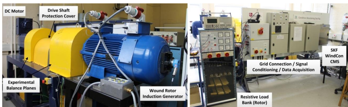
Figure 4.4: Durham WTCMTR without gearbox: main components, instrumentation and control systems.
