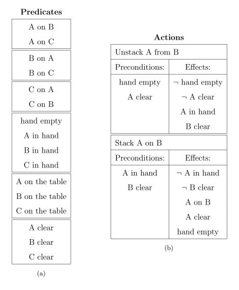
Table 4.1: (a) All possible Propositions for a 3 block Blocks World problem. (b) Example actions from the Blocks World domain. Preconditions are required to be true in a world state for an action to be applicable. The effects are the changes to propositions resulting from applying an action. Other actions are required for each pair of blocks, and actions for picking up blocks from the table and putting blocks down on the table.
