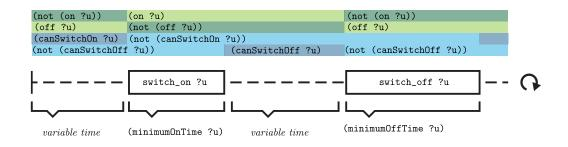
Figure 5.2: The two actions switch\_on and switch\_off can be scheduled to give any length online and offline periods despite having fixed duration. The temporal constraints are enforced using the predicates canSwitchOn and canSwitchOff.
