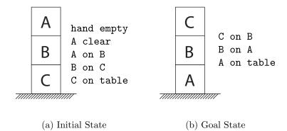
Figure 4.2: Figure illustrating a Blocks World problem with a valid initial state, which describes the state in its entirety, and a goal state which specifies facts which must be true, but does not require full specification of the state.
