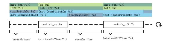
Figure 6.2: The two actions switch\_on and switch\_off can be scheduled to give any length online and offline periods despite having fixed duration. The temporal constraints are enforced using the predicates canSwitchOn and canSwitchOff
