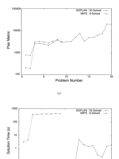
Figure 4.6: Results for the Temporal-Metric variant of the Openstacks domain from IPC 5. Results show that clearly SGPLAN has an advantage but if it is not performing the correct optimisation (as discussed in the main body text) then this performance could be misleading, implying planning performance on temporal-metric domains lags behind purely temporal domains. May 8, 2014
