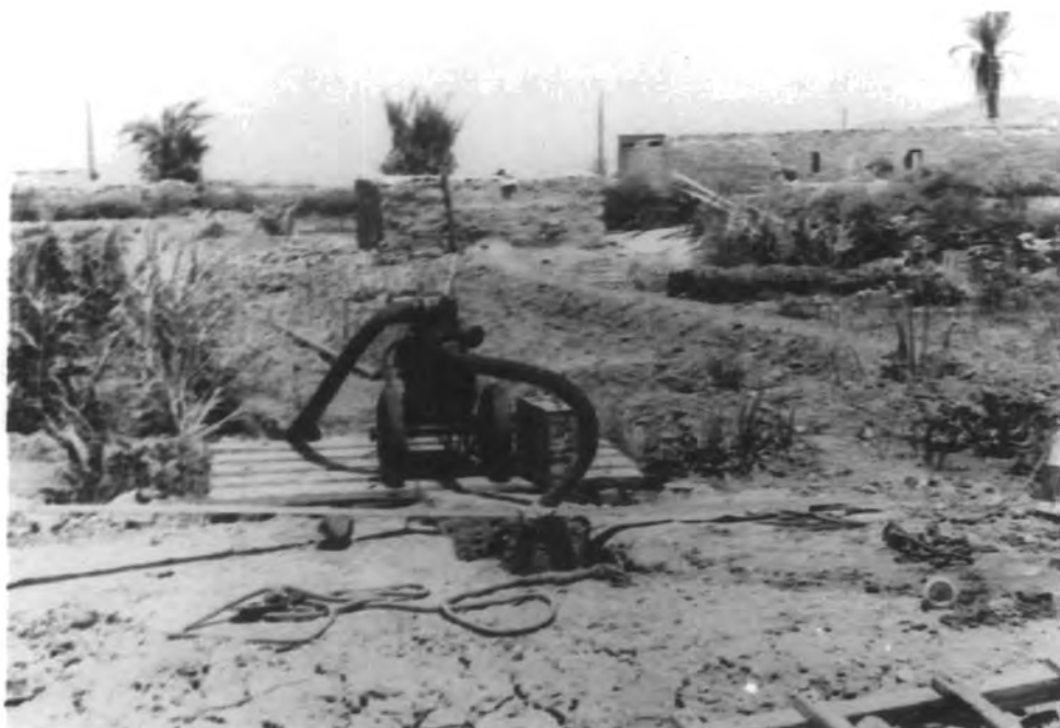
Plate 5.4. Portable engine pump at Sidi Abdalla, west of Tolmeita.
