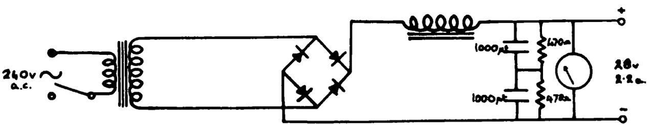
constructed low voltage d.c. power unit which supplies the Head Units. The circuit shows the orthodox arrangement of a power transformer and metal rectifier to give 28v, 2.2A unstabilised output.
