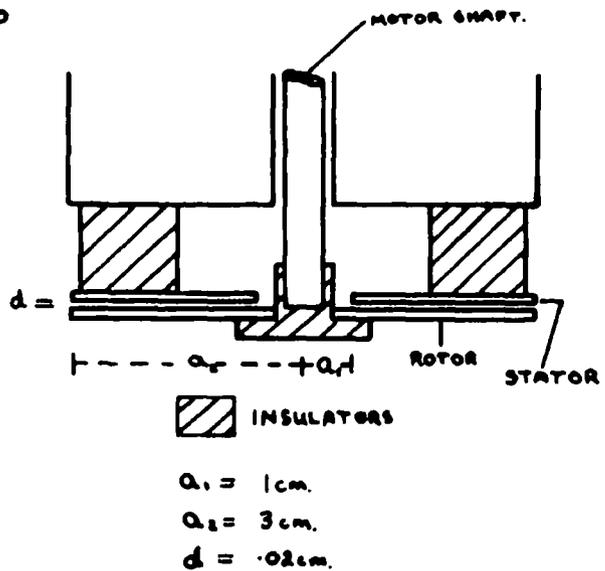
Fig.8 The Reference Generator - Construction.
