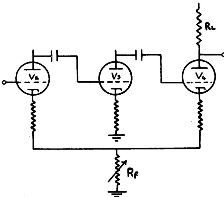
Fig. 12 The Amplifier - Simplified Circuit.
