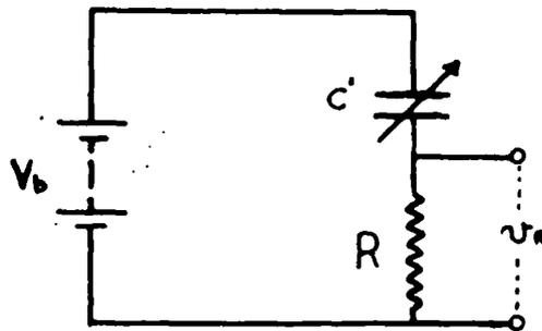
Fig.7 The Reference Generator - Equiv. Circuit.
