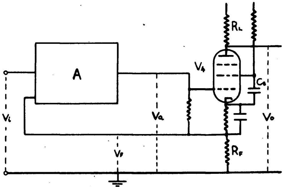
Fig.6 The Inclusion of the Schuster Circuit
