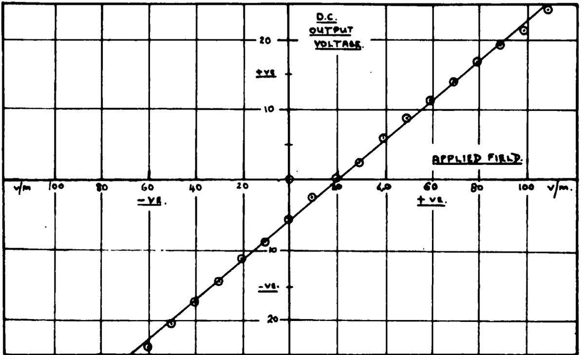
Fig. 16 A Mill Calibration Curve.
