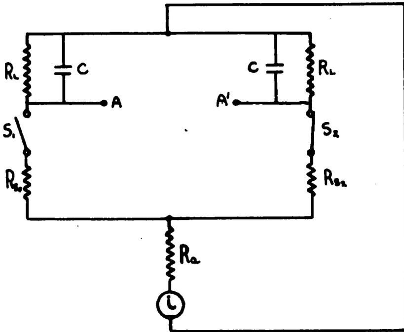
Fig.4 The Schuster Circuit - Equiv. Diagram.
