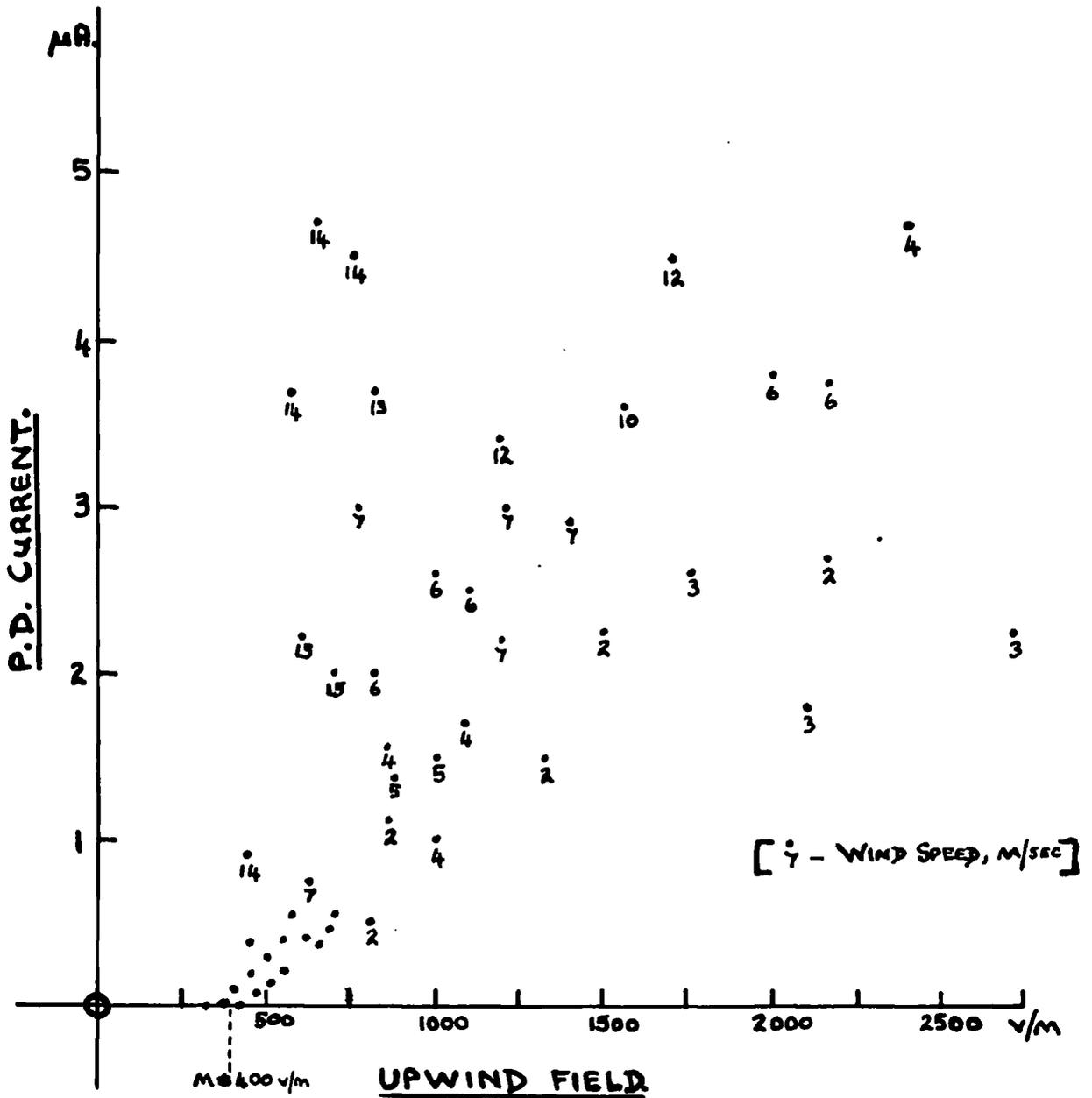
Fig. 21 Variation of Point Discharge Current with Field and Wind Speed.
