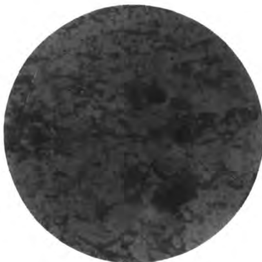
Fig.6.(R.J.93) Contact hornfels. North of the granite. A cordierite-quartz-albite-biotite hornfels. Probably a metamorphosed tuff. (x 35).
