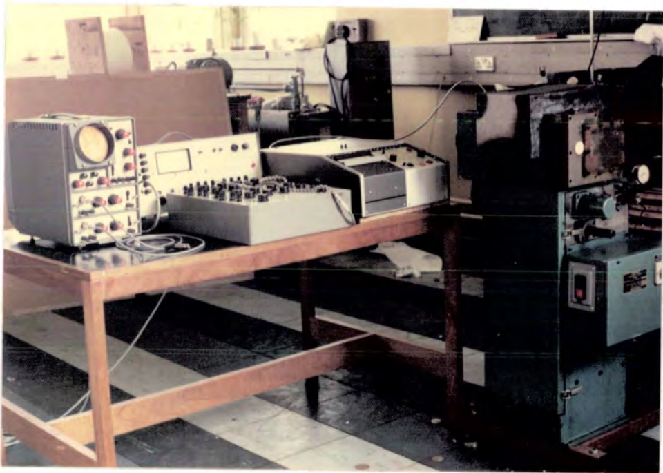
Plate 4.1 Oscilloscope, amplifier, switch box, u.v. recorder (with speed pick-up connection)
