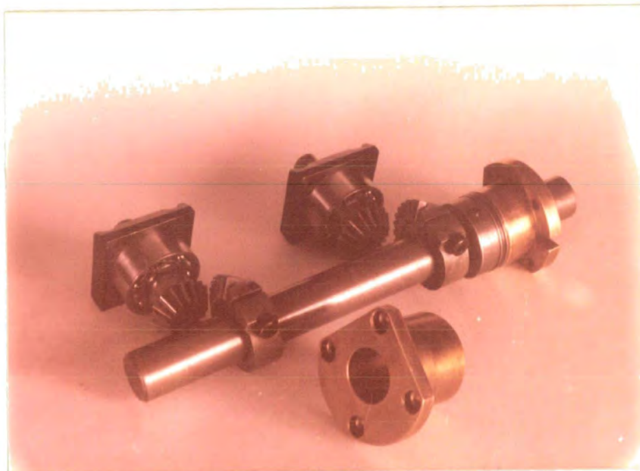
Plate 1.8 Shaft O_2 , shaft bearings, and the bevel gears.
