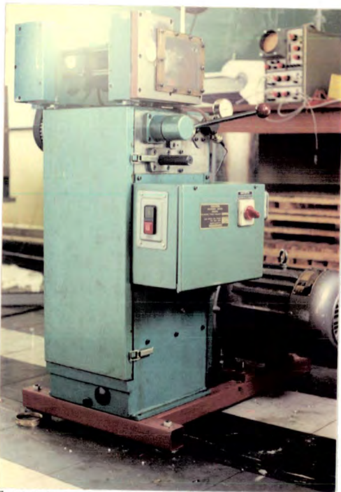
Plate 4.2 Featuring the viewing window modified to accept the strain gauge leads
