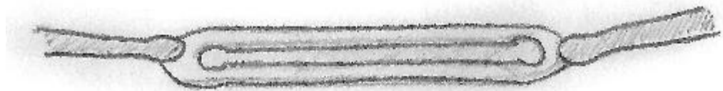
Fig. 2. An illustration of the drawing method of glass bead manufacture. A tube of molten glass is drawn out, before individual beads are produced and severed from it.
