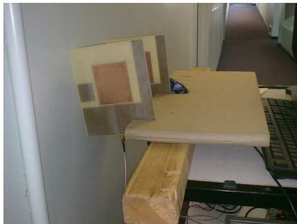
Figure 5.9 Patch-like antennas close to a brick wall
