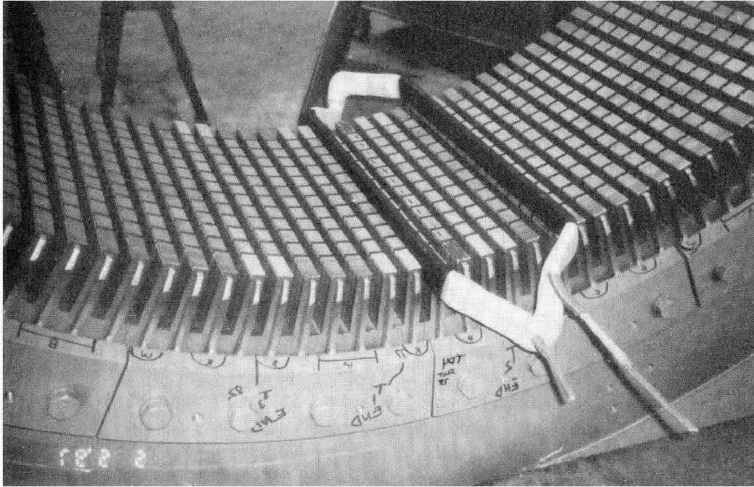
Figure 4.2: Form-wound stator winding, reproduced from [16]
