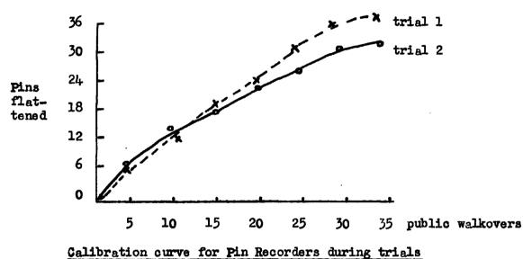
On this pattern the reliability of recording could give comparable results for any path. It was not able to compare between paths, owing to the different stages at which falling away on the calibration curve was reached, and this was related to the width of the path, and in some instances, to the degree of public pressure.
