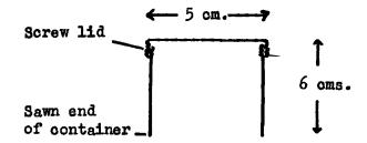
With this apparatus soil cores could be easily removed without disruption by removing the lid and gently loosening. The first 3 cms. was considered more important and after cutting to this length, the samples were weighed, placed in an oven at  $80^{\circ}$ C for 48 hours and reweighed on cooling.
