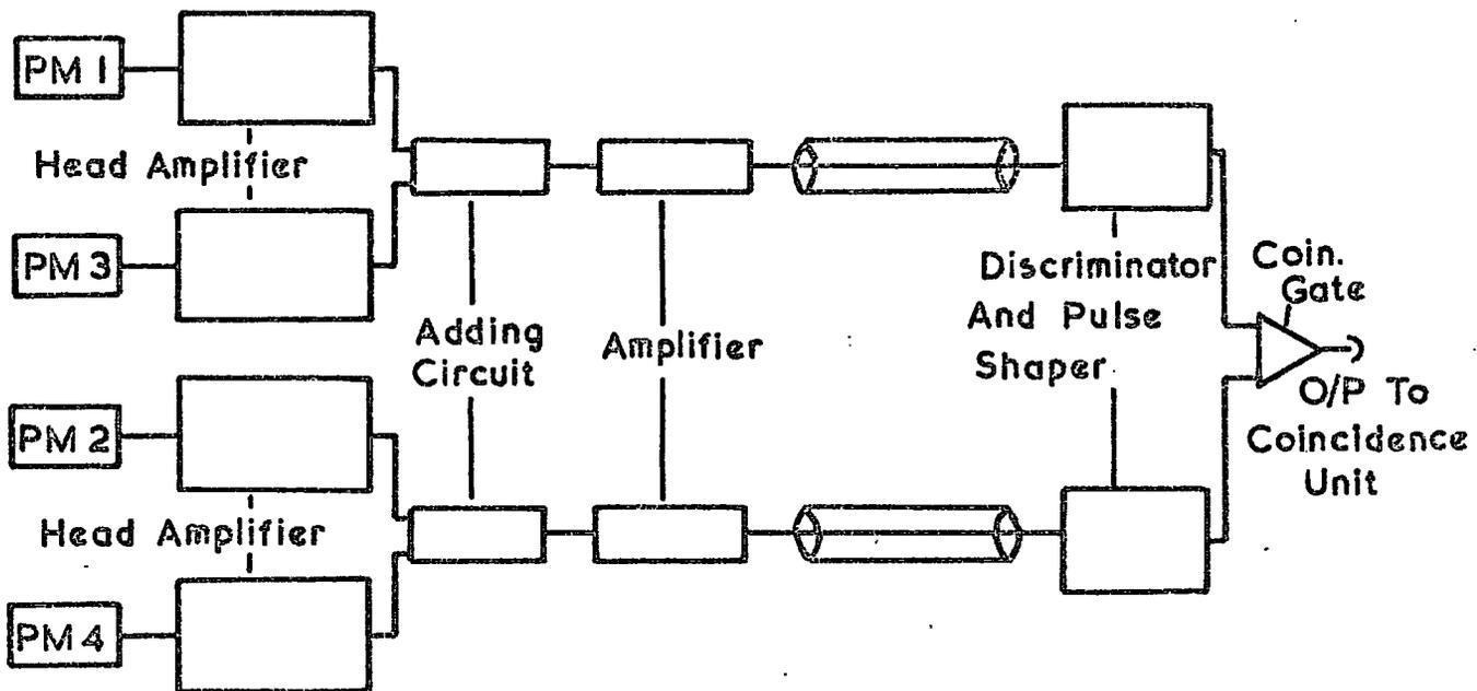
Figure 3.5 Block diagram of the electronics for the scintillation counter
