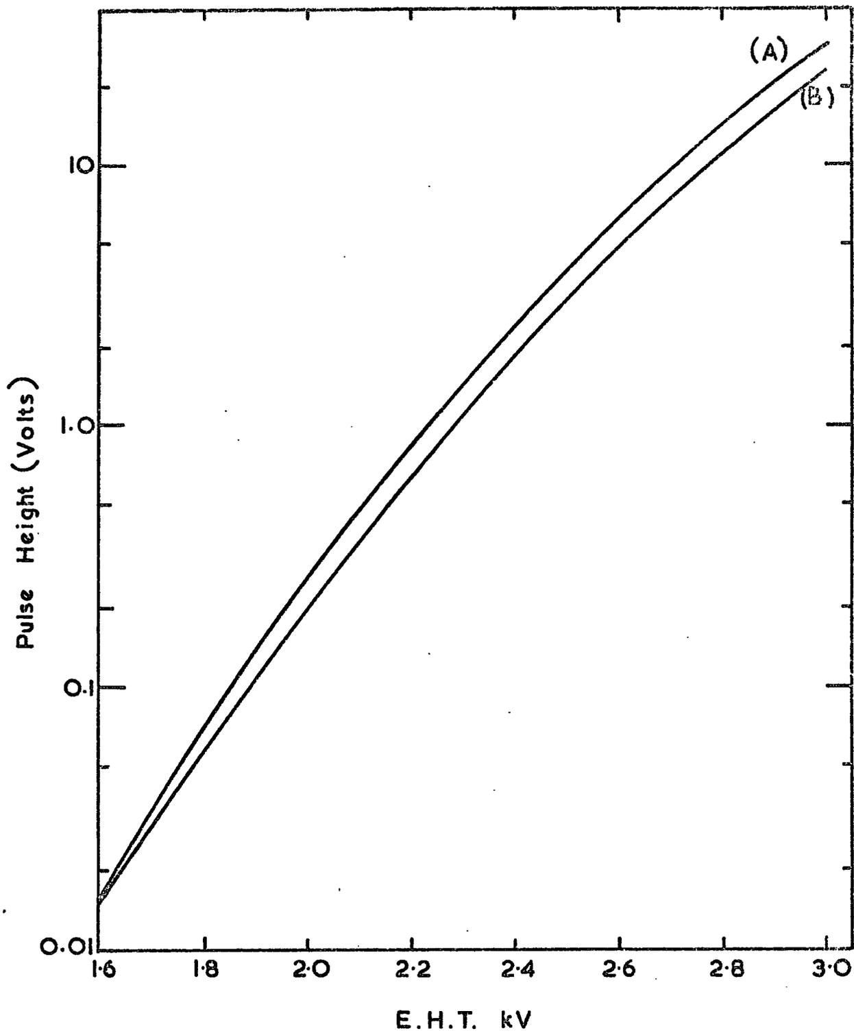
Figure 5.2 Variation of gain with E.H.T. for the two extra photomultipliers on S1
