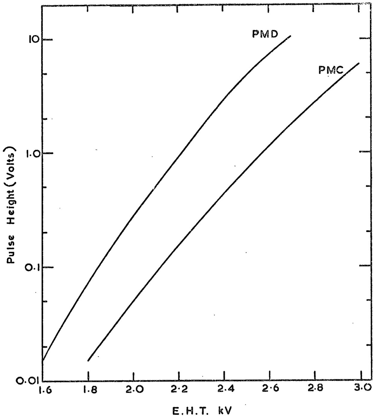
Figure 5.3 Variation of gain with E.H.T. for the two extra photomultipliers on S3
