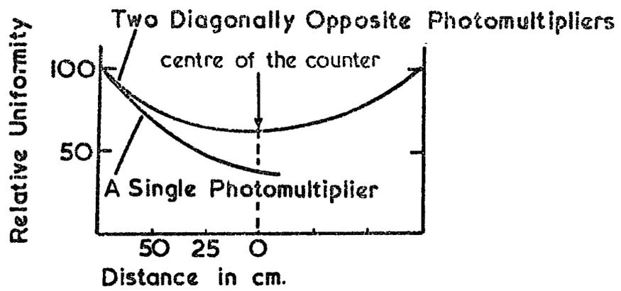
Figure 3.4 The uniformity of the scintillation counter
