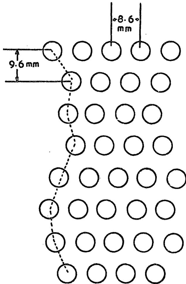
Figure 3.6 The pattern of flash tubes in the measuring tray
