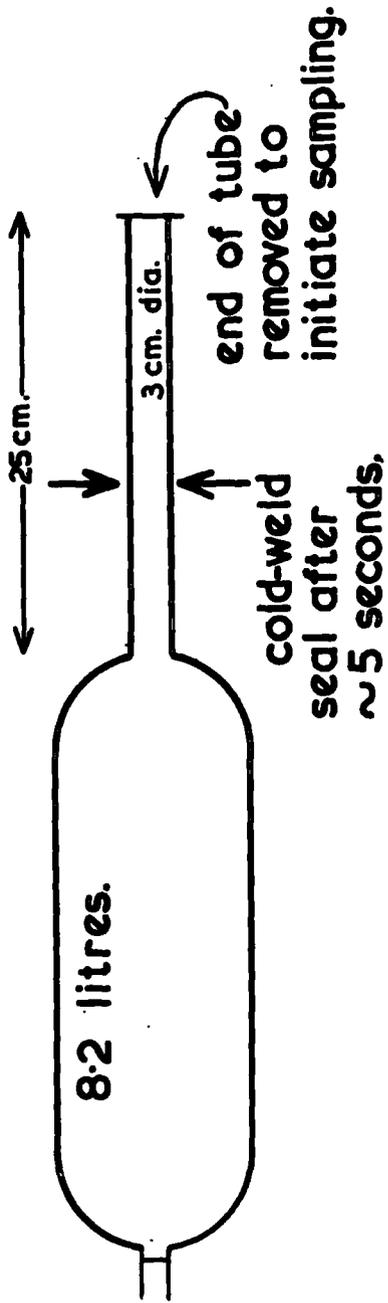
Impedance of inlet tube  $\sim 0.1$  second / litre under molecular flow conditions; effectively less at higher pressures.
