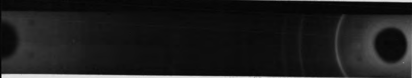
FIGURE 6.4.7 X-ray diffraction photograph of milled (cubic) CdSe
