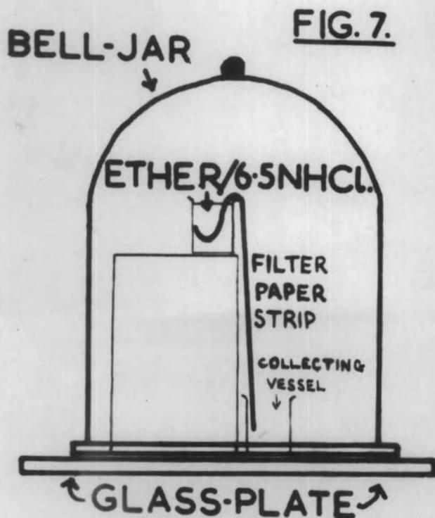
quantitative recoveries in micro-analytical work, the ideal separation would be one in which the substance being studied remained stationary on the column or paper strip, while the other substances were removed by the solvent flow.
