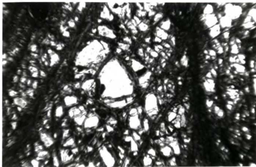
Plate 16 Olivine with serpentinised rims (X20).
