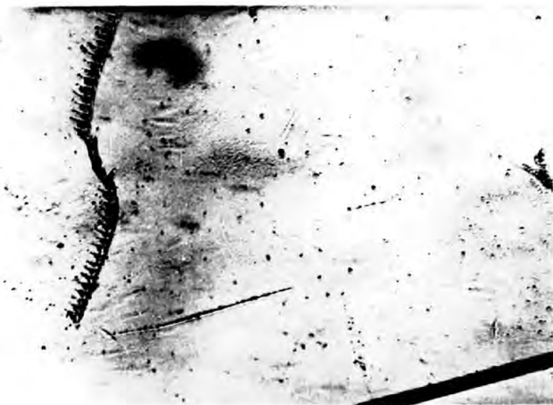
A compressive stress of 0.7 \text{ kgms/mm}^2 has been applied along the [010] direction. The direction of stress is indicated by the black line.
