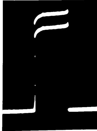
A. Trace of a square pulse recorded through a 10 megohm resistor in place of an electrode. Superimposed is a pulse recorded through the same when a 20 megohm shunt is switched across the inputs.
