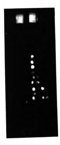
Single Ionising Particle Knock-on Electrons produced in the Tube Assembly
