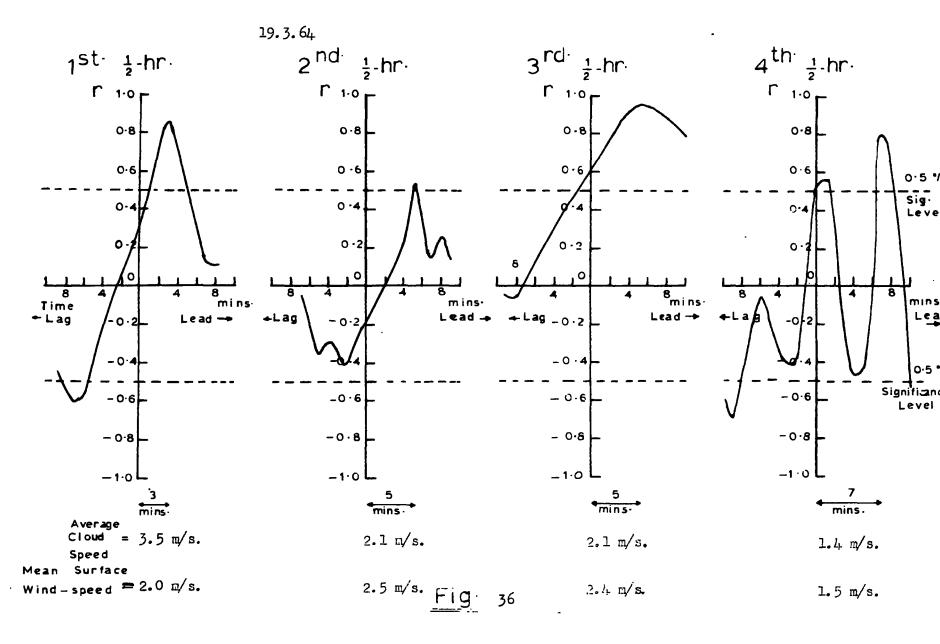
Figs. 36, 37: Graphs of correlation coefficients between snow currents measured at the Laboratory and Observatory against time-lag (and lead) of the former on the latter.
