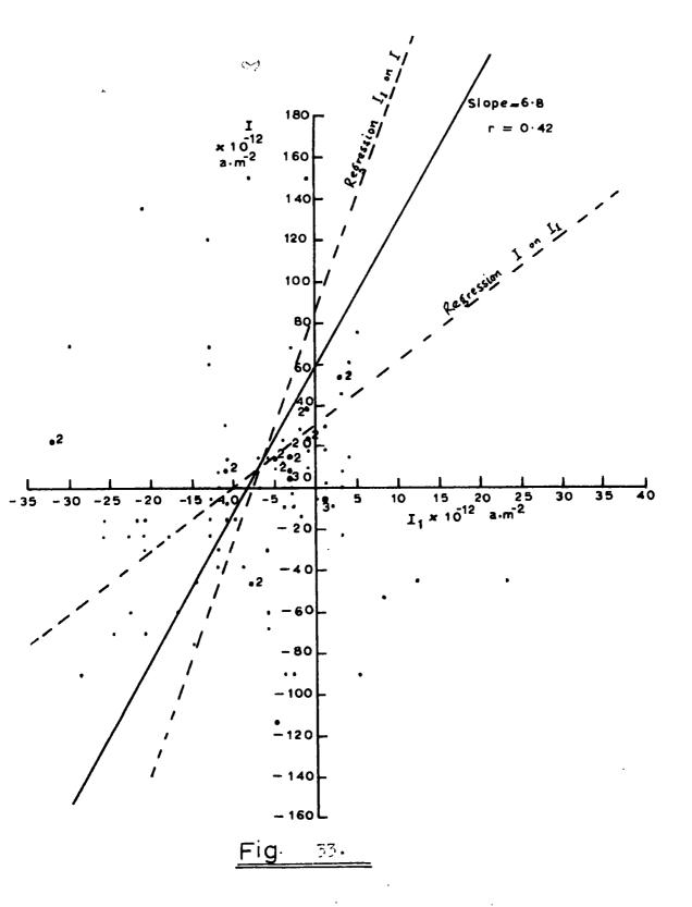
Simultaneous readings of snow currents to two receivers, 900 m. apart. (I<sub>2</sub> at top of mast).
