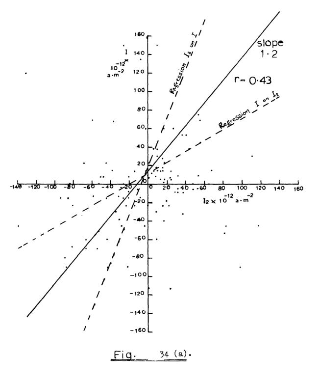
Snow currents to two receivers, 900 m. apart: 7 mins. time-lag of  $I_2$  (at top of mast) on I.
