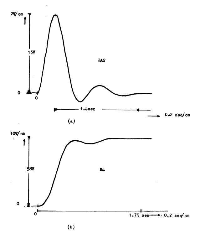
Figure 4.6 Response of the mathematical governor model to -26.25 step input
