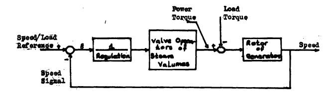
Figure 1.8 Block diagram of speed central leep
