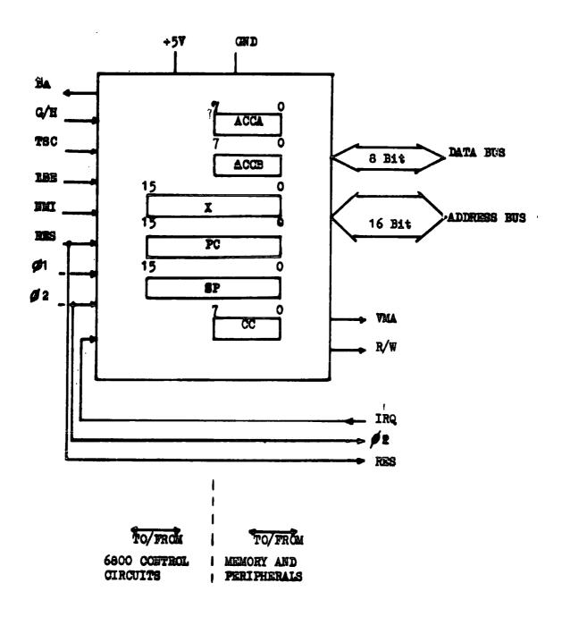
Figure 3.2 MC6800 Microprocessing Unit
