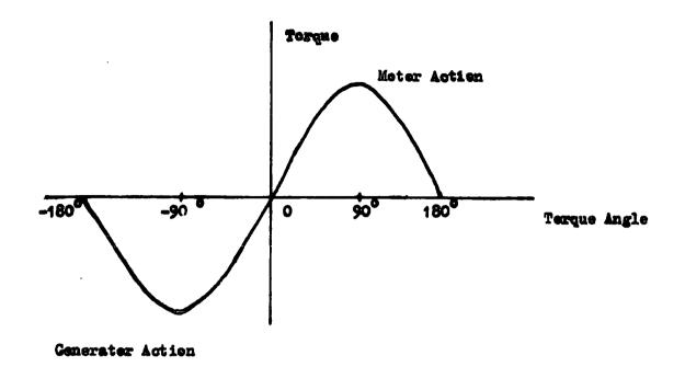
Figure 1.1 Temque-Angle Curve of a Synchronous Machine
