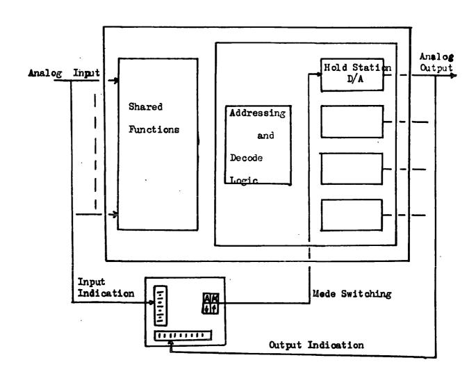
Figure 2.5 Display back-up system
