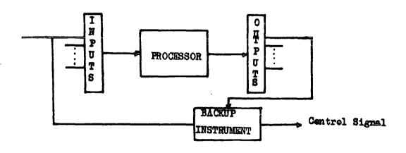
Figure 2.4 Manually backed-up system
