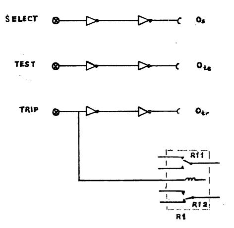
Figure 5.3 Pushbutten connections.
