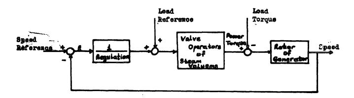
Mgare 1.9 Block diagram of "Separate Speed and Lead"
