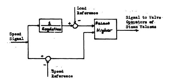
Figure 1.10 Block diagram of "Speed and Lead Centrel by
