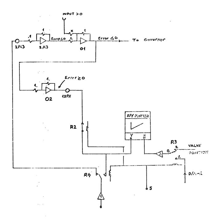
Figure 6.1 Hardware configuration for the simulation of the ramp signal addition procedure.
