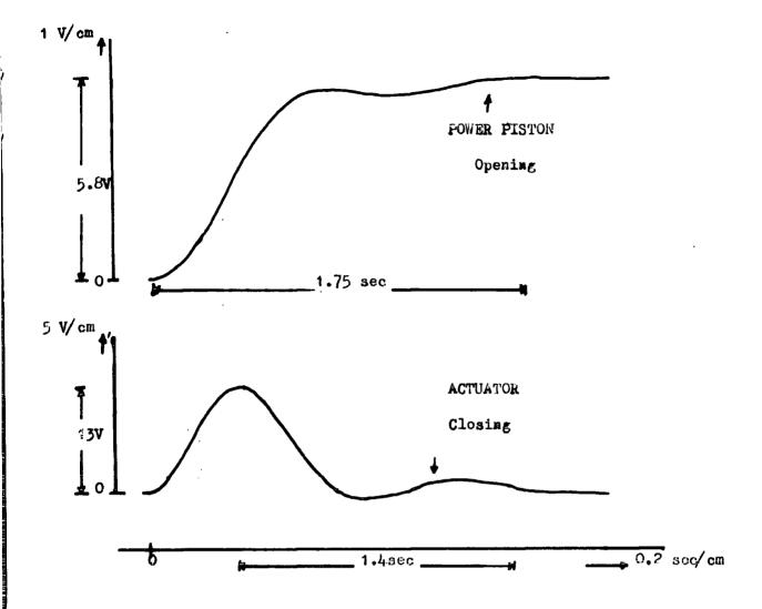
Figure 4.5 Power Pistom response in opening direction and
