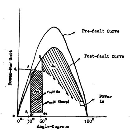
Figure 1.6 Transient-stability imprevement by fast valve action.
