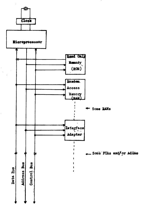
Figure 3.1 M6800 Microcomputer family block diagram
