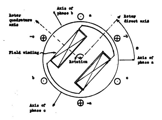
Figure 1.2 Elementary salient-pole 3-phase synchronous machine
