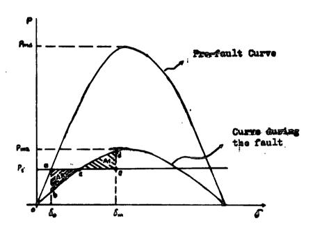
Figure 1.5 Determination of stability limit by the equal-area criterion.
