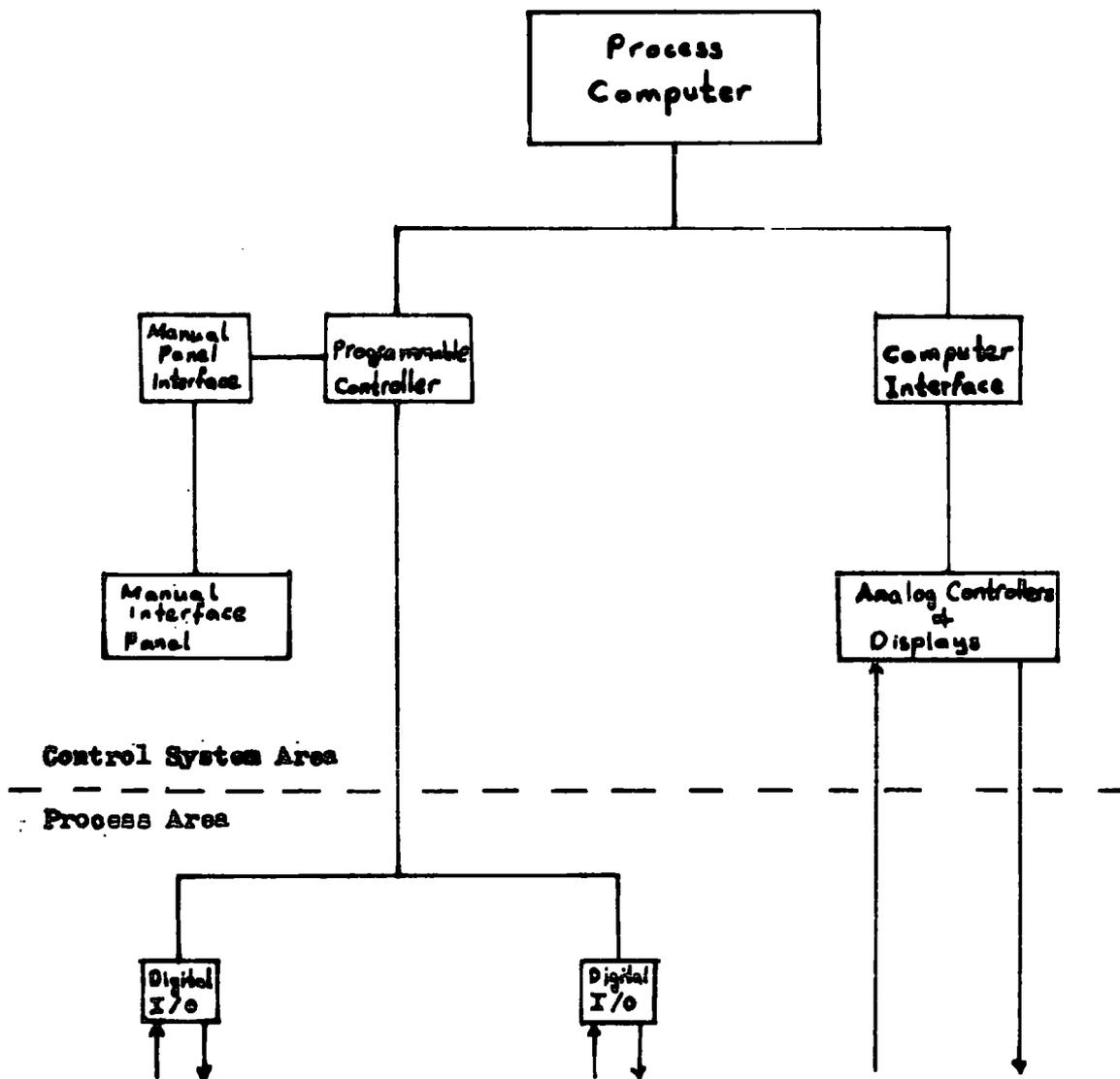
Figure 2.6 An on-line computer control system with two computers connected in series.
