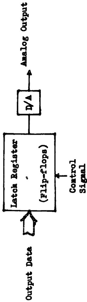
Figure 2.2 'Latching Parallel Data' system
