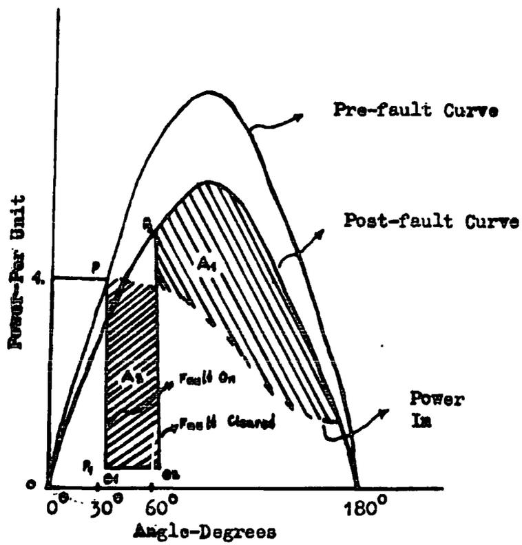
Figure 1.6 Transient-stability improvement by fast valve action.
