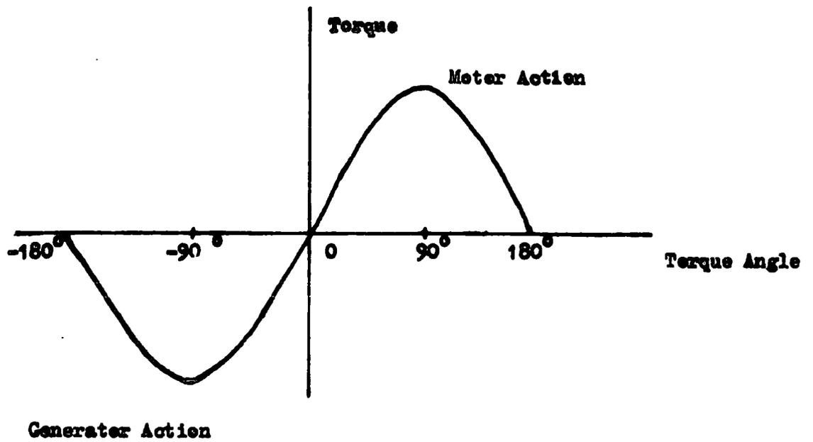
Figure 1.1 Torque-Angle Curve of a Synchronous Machine
