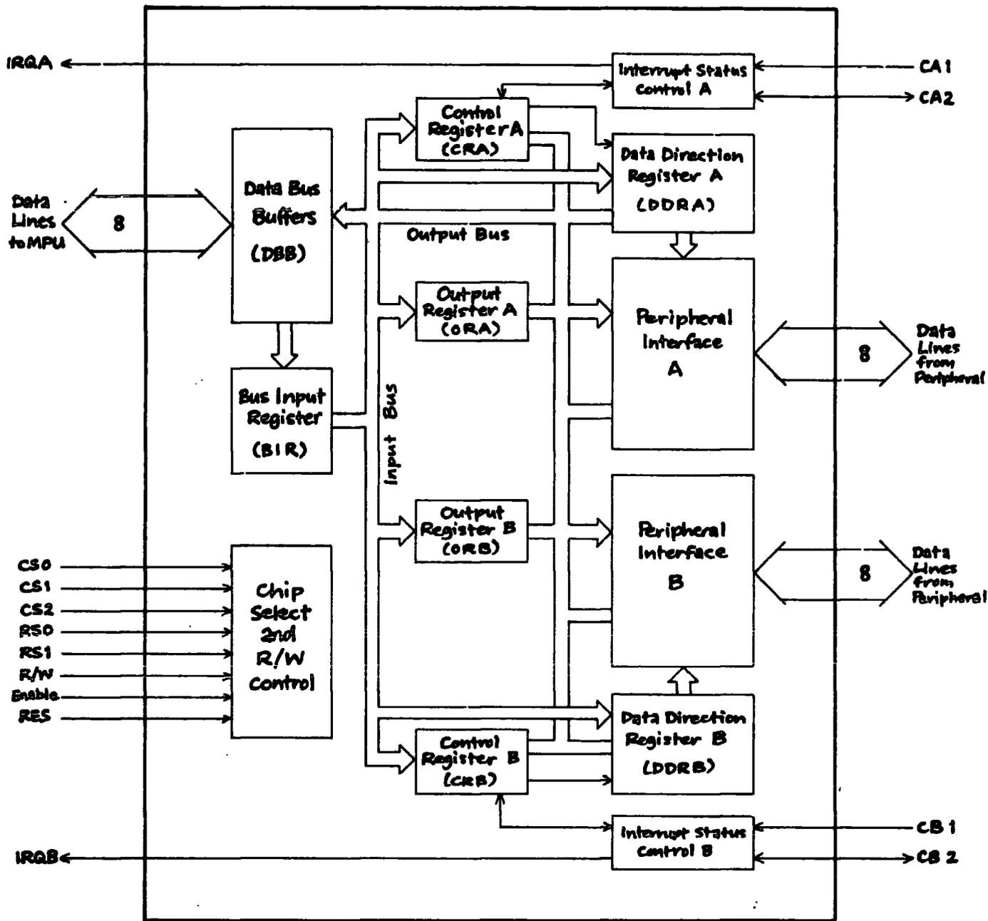
Figure 3.3 The expanded block diagram of MC 6820 Peripheral Interface Adapter
