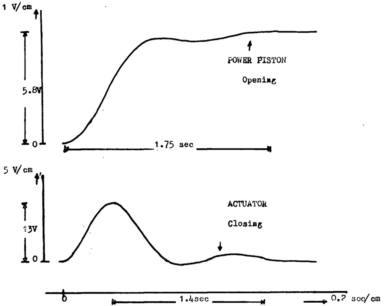
Figure 4.5 Power Piston response in opening direction and Actuator response in closing direction to -26.25 volt step input
