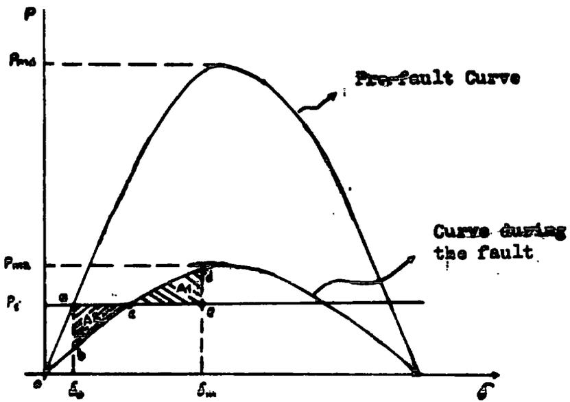
Figure 1.5 Determination of stability limit by the equal-area criterion.
