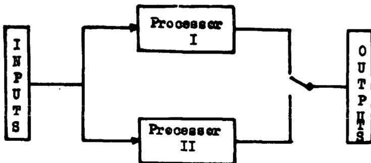
Figure 2.3 'Multiple processors' method
