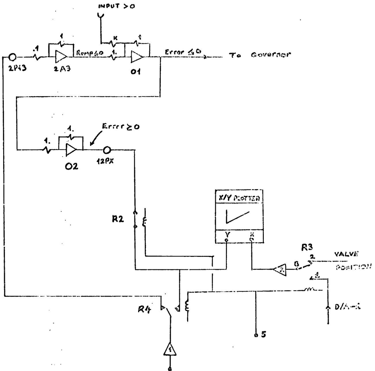
Figure 6.1 Hardware configuration for the simulation of the ramp signal addition procedure.
