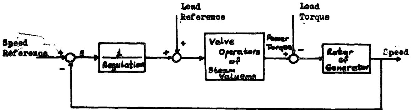
Figure 1.9 Block diagram of "Separate Speed and Load" controls for an electro-hydraulic control system.
