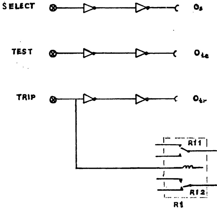
Figure 5.3 Pushbutton connections.
