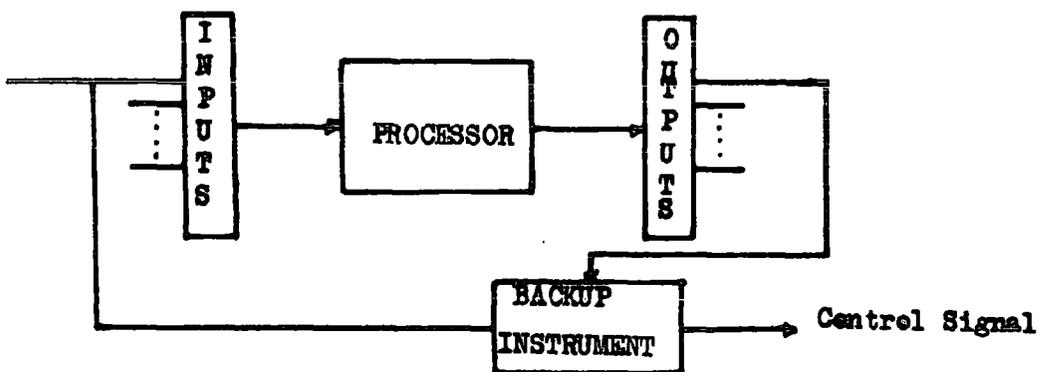
Figure 2.4 Manually backed-up system
