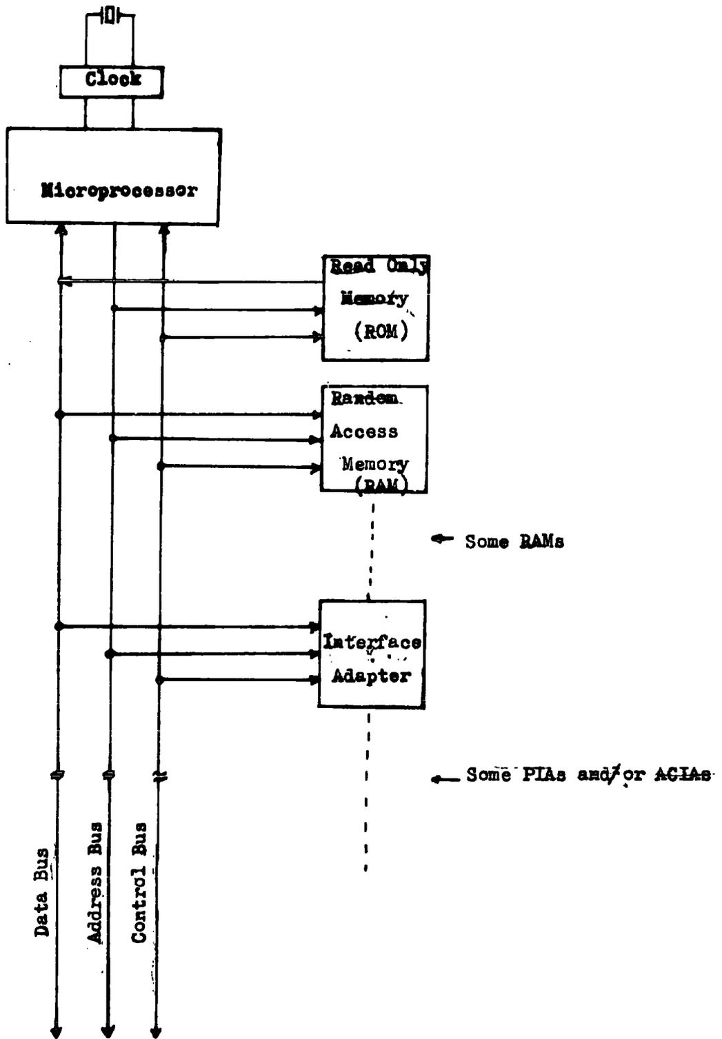
Figure 3.1 M6800 Microcomputer family block diagram
