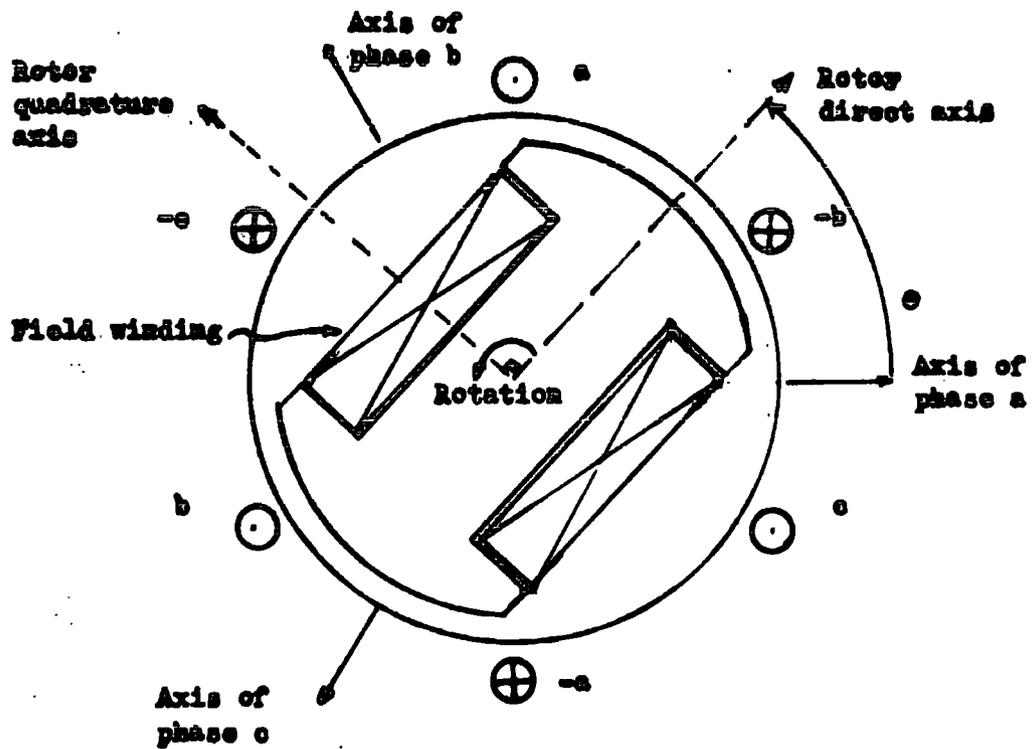
Figure 1.2 Elementary salient-pole 3-phase synchronous machine
