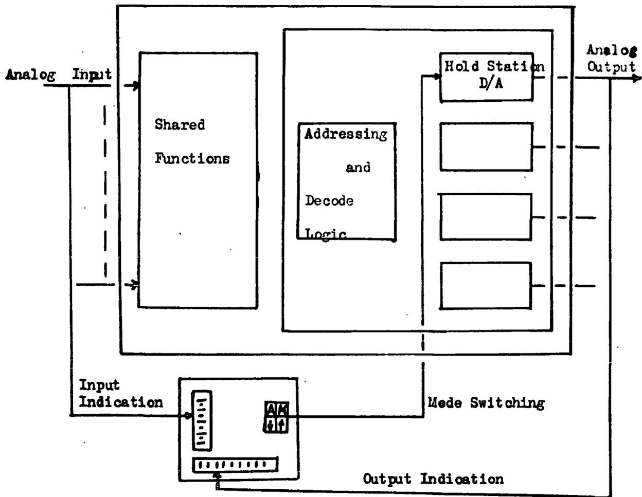
Figure 2.5 Display back-up system
