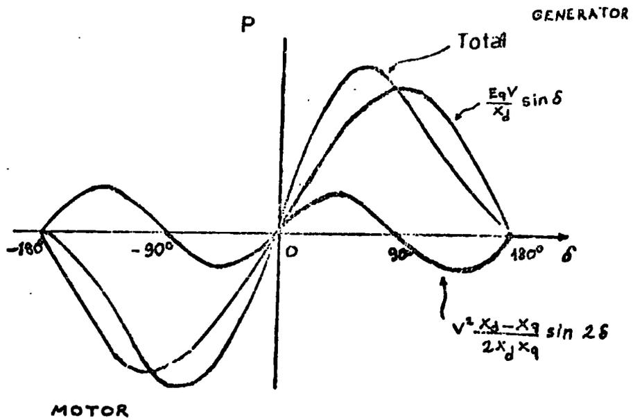
Figure 1.3 Steady-state power-angle curve of salient-pole synchronous machine.
