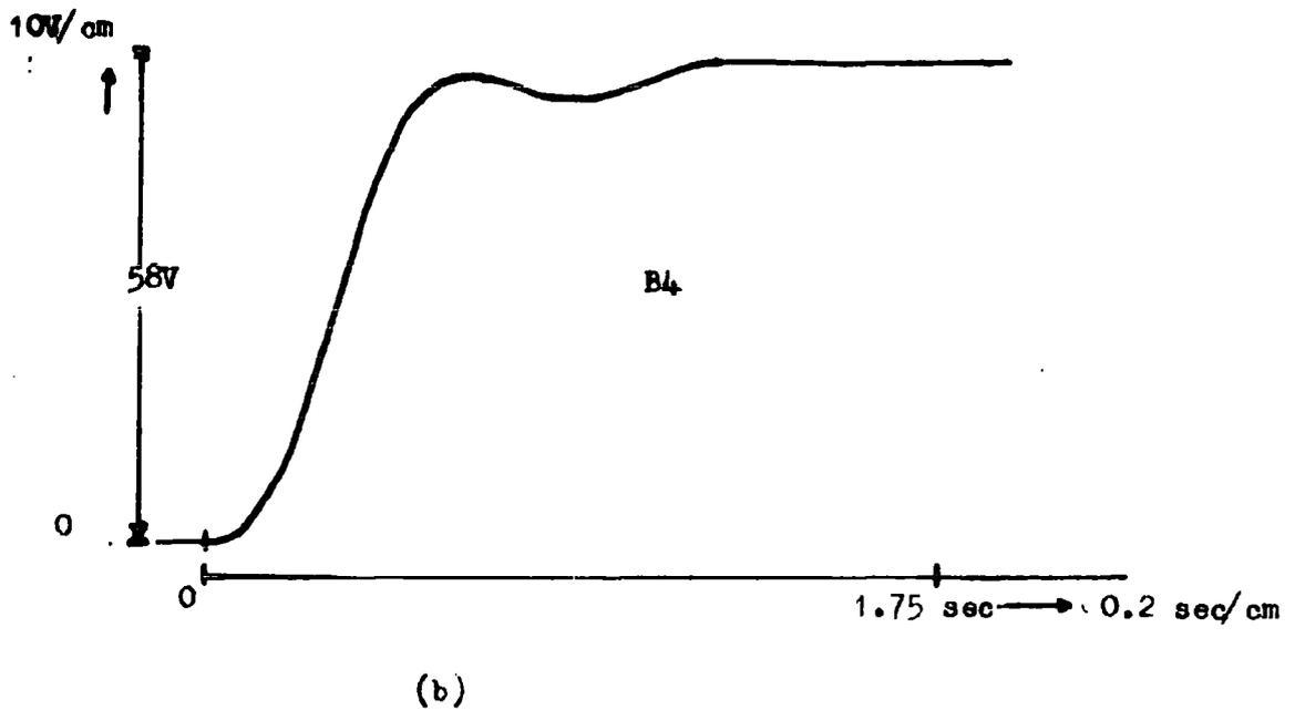
Figure 4.6 Response of the mathematical governor model to  $-26.25^{\circ}$  step input
