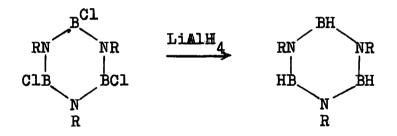
Since the B-trichloro-N-substituted borazines are fairly readily accessible from boron trichloride and the appropriate amine hydrochloride B-N substituted borazines are also readily prepared from the B-trichloro compounds and Grignard or organo lithium reagents,<sup>82</sup> or by Friedel-Craft arylation.<sup>83</sup>
