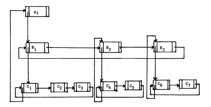
FIG. 2.19. CHAIN AND RING STRUCTURE.
