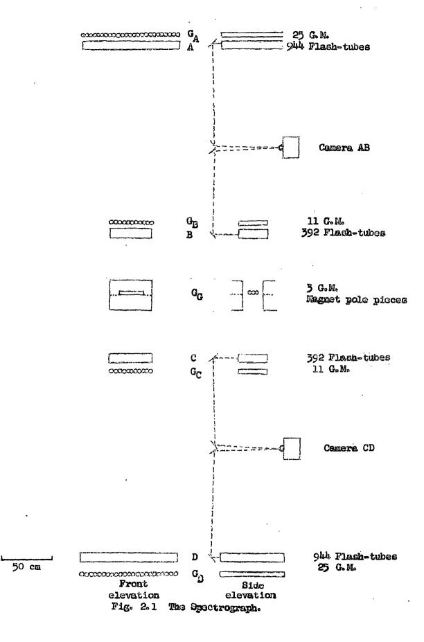
counters. All the counters in the trays at A, B, C and D are positioned with their axes parallel to the magnetic field. The tray at level G consists of three 26 cm long counters with their axes at  $90^{\circ}$  to the magnetic field. The counters are of the selfquenching type (20th Century G26, G60) but in order to reduce their dead-time, the discharge is also quenched electronically. The electronic circuits used with the Geiger counters are described fully by Jones et al., (1962).
