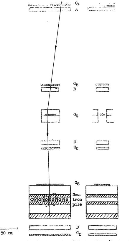
The Spectrograph and Neutron Pile (E, S and P Series)
