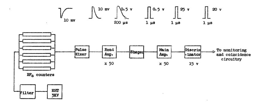
Block Diegram of Neutron Recording Circuitry
