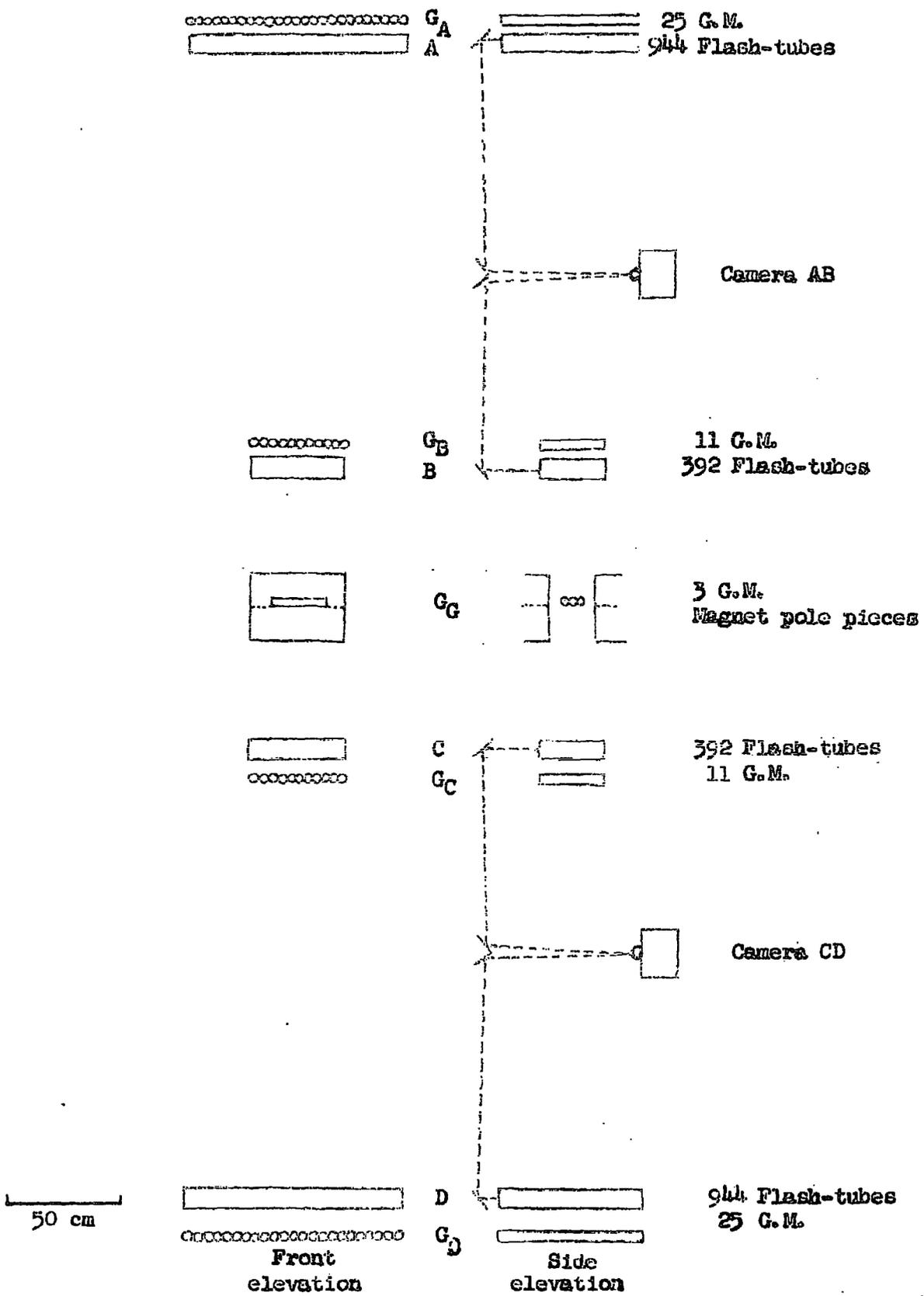
Fig. 2.1 The Spectrograph.
