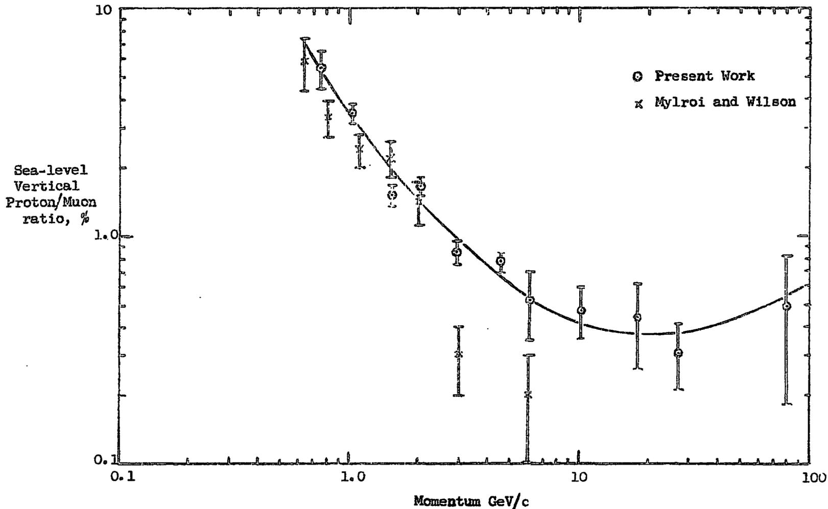
The Sea-Level Proton/Muon Ratio as a Function of Momentum
