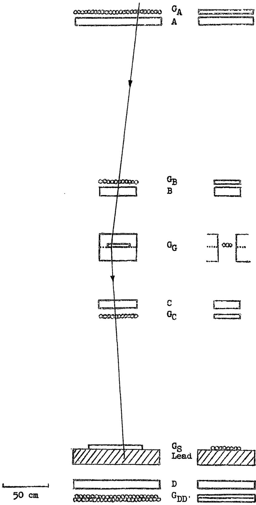
The Spectrograph and Lead Absorber (AP Series)
