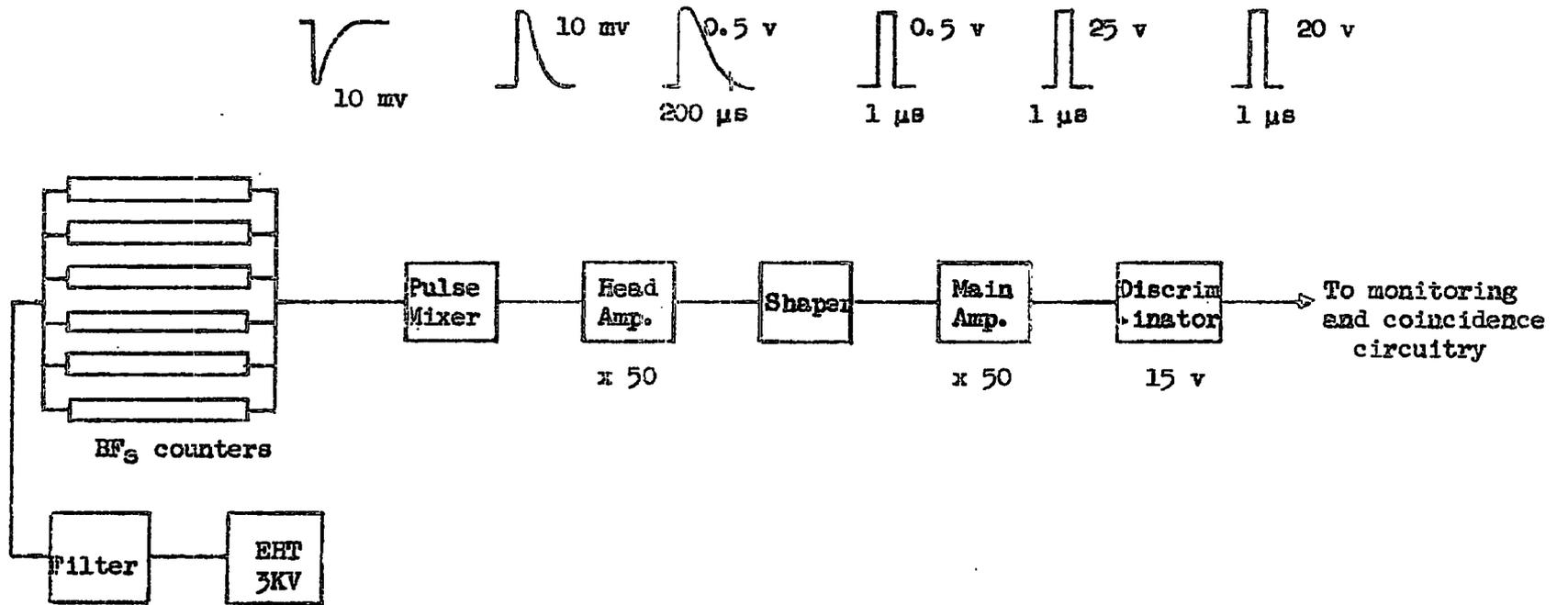
Block Diagram of Neutron Recording Circuitry
