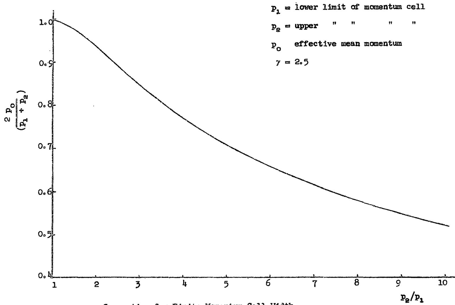
Correction for Finite Momentum Cell Width
