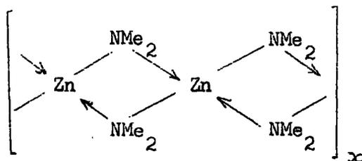
Evidently the donor character of the dimethylamino-group when bound to zinc is so enhanced that even bipyridyl causes no displacement. An attempted preparation of  $(\text{Me}_2\text{N})_2\text{Zn}$  bipy from the dimethylzinc complex,  $\text{Me}_2\text{Zn}$  bipy and dimethylamine at 80°, yielded only black, involatile and insoluble material in addition to methane. It is not known whether the bisamino-compound is formed by disproportionation of
