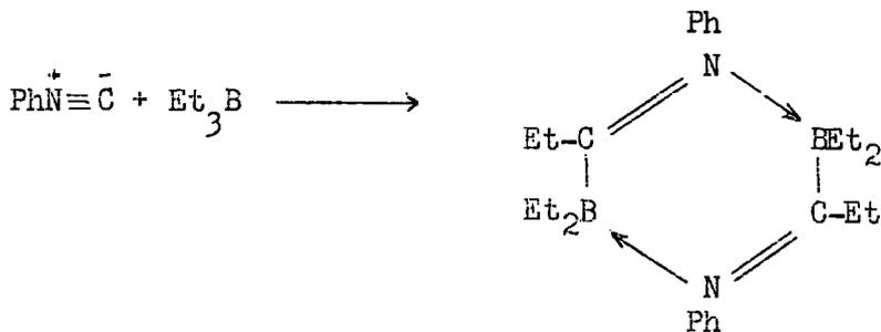
A similar compound has been obtained by reaction of triethylboron with ethylisocyanide,<sup>142</sup> although trimethylboron and t-butyliisocyanide yield, rather surprisingly, the monomer  $\text{Me}_3\text{CN}=\text{CMe}\cdot\text{BMe}_2$ .<sup>143</sup>
