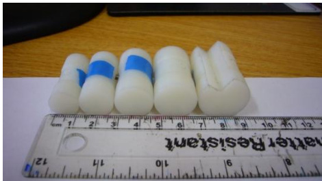
Fig. 7.3 The cylindrical rods used to estimate the bending radius of curvature of the device.
