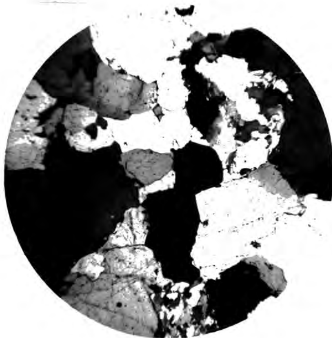
Fig. 34. Moderately sorted coarse to very coarse grained sandstone with polycrystalline grains and secondary overgrowths; High Coal Sill major washout-channel sandstone base, Sunny Brow Mine Quarry, near St. John's Chapel. Crossed nicols, x 27.
