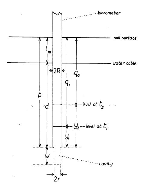
Fig. 3.21 Diagram to illustrate method of determining hydraulic conductivity of peat by means of a piezometer tube.
