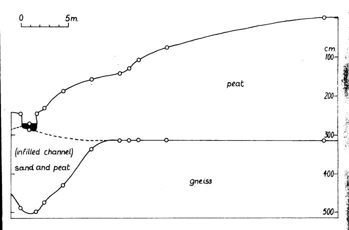
Fig. 3.3 Section through peat deposit at Tarraigheal, following the line of Transect "A". Levelled April 1963.
