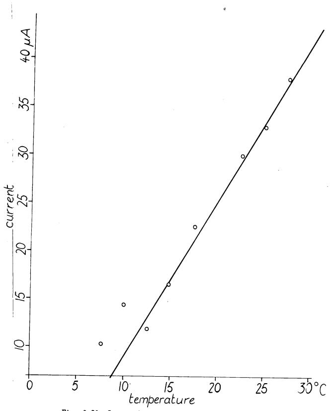
Fig. 3.20 Curve of diffusion current and temperature at constant oxygen concentration, the current corrected to 100umho. Rotating electrode.
