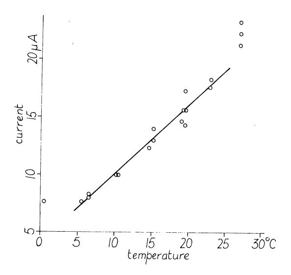
Fig. 3.17 Curve of diffusion current and temperature at constant oxygen concentration, without conductivity correction. Stationary electrode.
